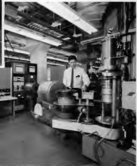
Left, 1949 oscillator at Graphite Reactor adapted from a Maytag washing machine for measuring neutron cross sections; right, neutron beam hole at HFIR.
