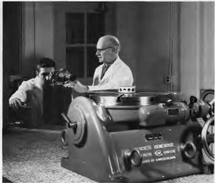
Apprentice training in optical evaluation of machine accuracy, H. Seaman instructing.
