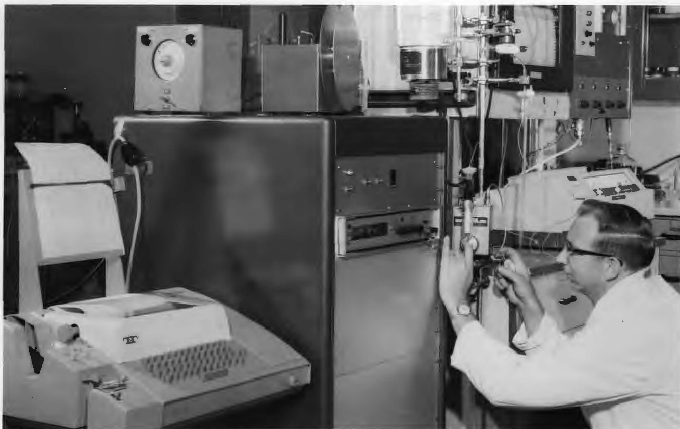
Norman Lee, technician from Chem Tech, adjusts the flow rate of the chromatographic system.
