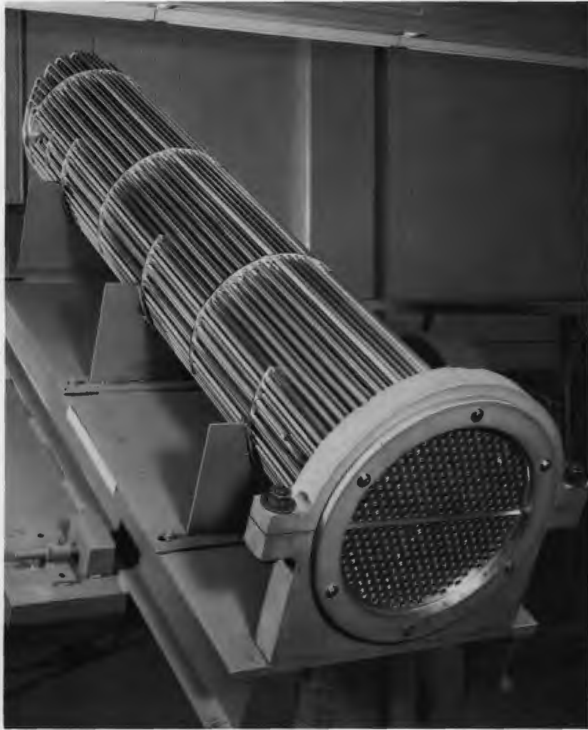
Figure 3. Completed tube bundle for the MSRE primary heat exchanger. The bundle consists of 163 half-inch OD tubes of INOR-8 joined to a 1½" thick header.
