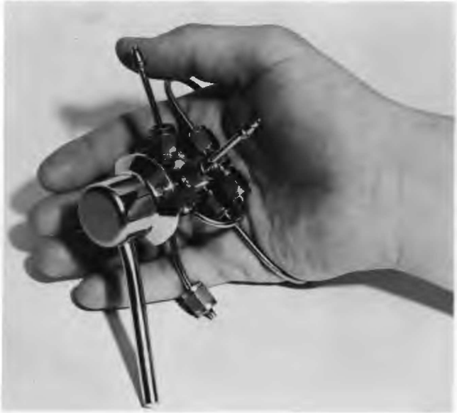
V. E. Walker of Instrumentation and Controls demonstrates the automatic injection valve he developed (shown above) with Scott and W. F. Johnson to inject controlled samples into the high-pressure stream of the analyzers.
