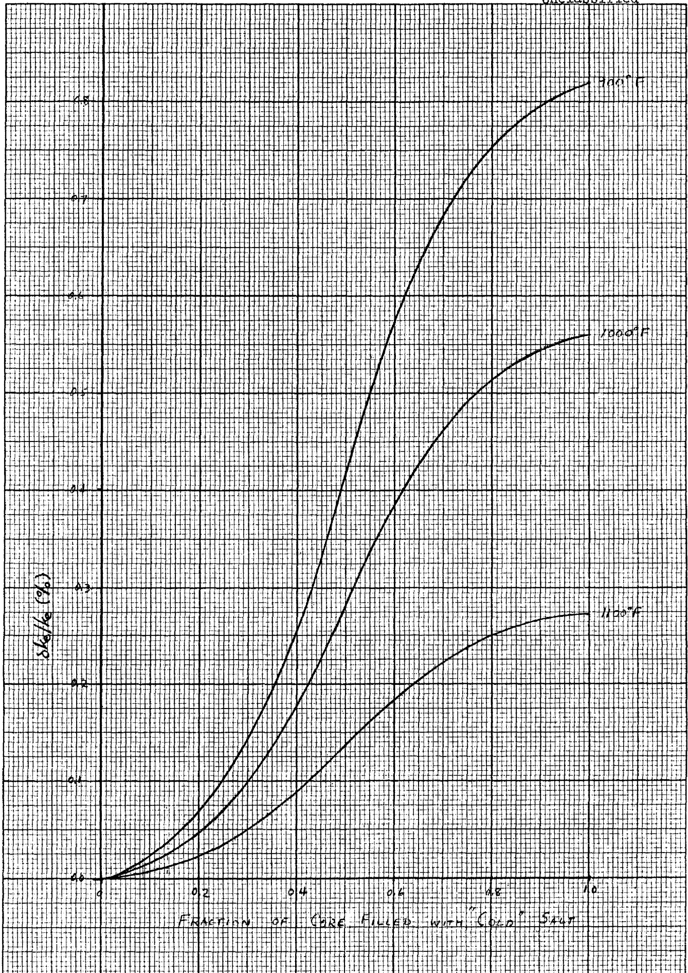
Fig A-4 Excess Reactivity Due to Replacing Part of Fuel in 1200° Core with Denser Fuel. (Fill from bottom up.)
