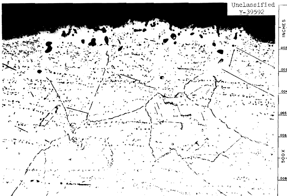
Fig. 12. Photomicrographs of a Type 304 Stainless Steel Specimen Tested in Tension at 75°F (25°C). (a) Gage section; (b) shoulder. Strain rate was 0.0125 in./in.-min. Prior to testing, specimen was (1) annealed for 1 hr at 1900°F (1038°C) in H 2 and (2) stressed at 3400 psi in CO 2 at 1500°F (816°C) for 1727 hr. Etchant: aqua regia. Reduced 21.5%.
