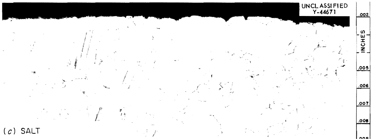
Fig. 25. Sections from 90 Ni-10 Co Specimen 21 from Group II Volatility Pilot Plant Fluorinator Test Specimens. Vapor section is as-polished. Interface and salt sections are as-etched with 92\text{HCl}:5\text{H}_2\text{SO}_4:3\text{HNO}_3 . 300X.
