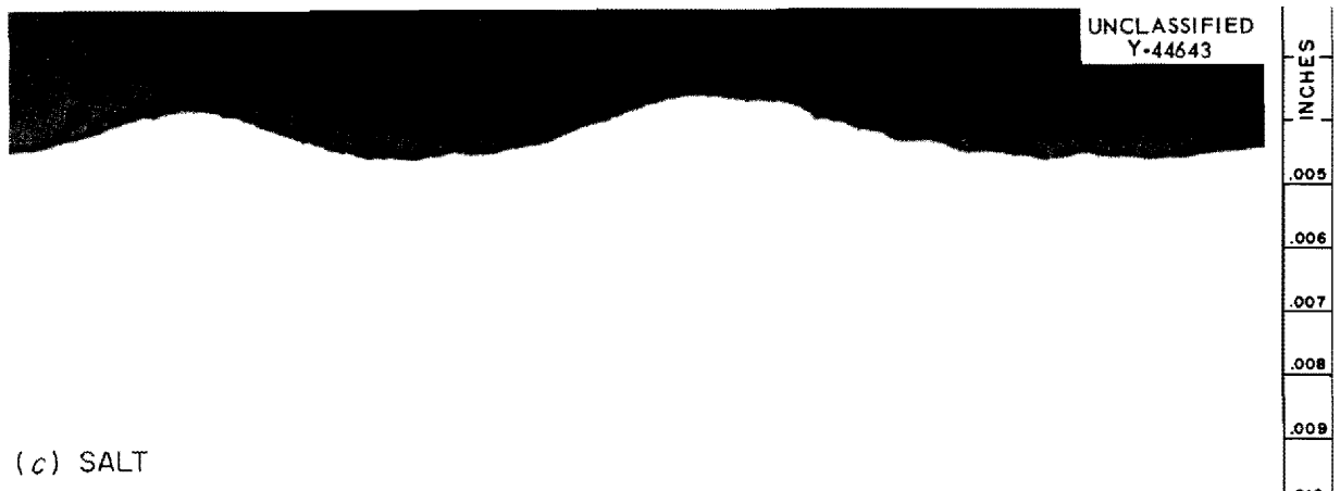
Fig. 23. Sections from INCO-61 Weld Deposits of Specimen 52 from Group II Volatility Pilot Plant Fluorinator Test Specimens. As-polished. 300X.
