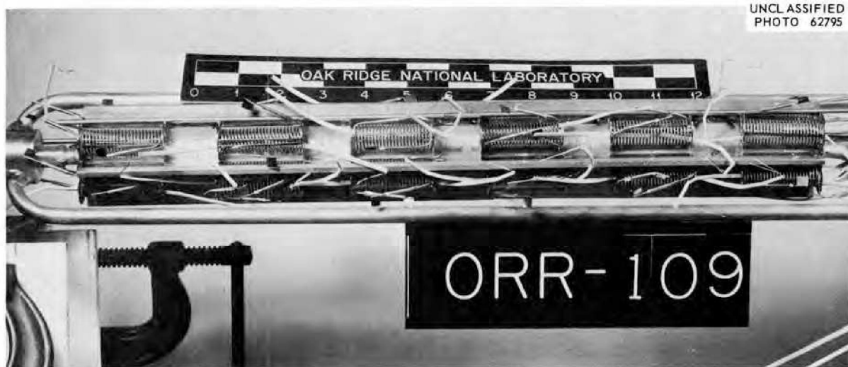
Fig. 1. Photograph of In-Reactor Irradiation Rig Showing Tensile Specimens in Furnaces.
