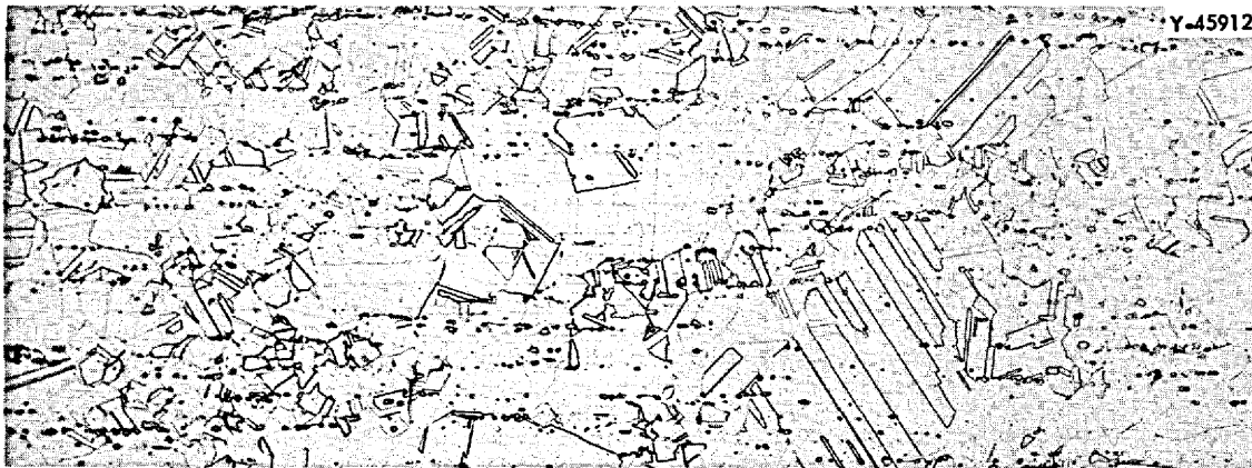
Fig. 2. As-Received INOR-8 Heat 5075. Etchant: aqua regia. 100X.
