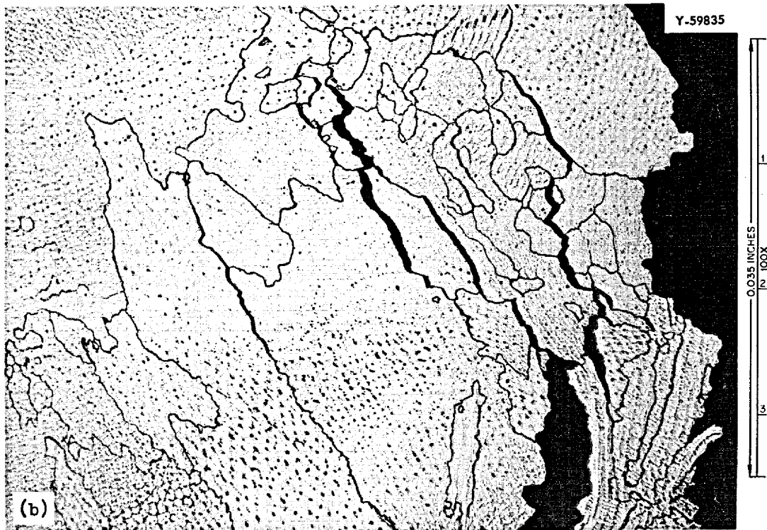
Fig. 16 - Creep-rupture failures of MSRE INOR-8 transverse weld specimens. A. Base metal failure in heat 5075, tested at 1100°F; applied stress 54,000 psi, rupture time 53.0 hr, total strain 1.4%. B. Weld metal failure in heat 5072, tested at 1300°F; applied stress 45,000 psi, rupture time 7.2 hr, total strain 7.5%. Etchant: CrO 3 , HCl, H 2 O. 100X.
