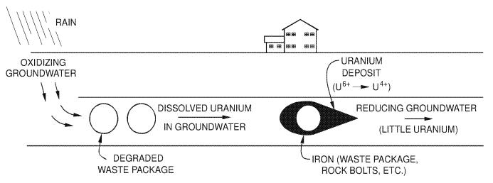
Fig. 2. Natural and man-made formation of uranium ore deposits.
