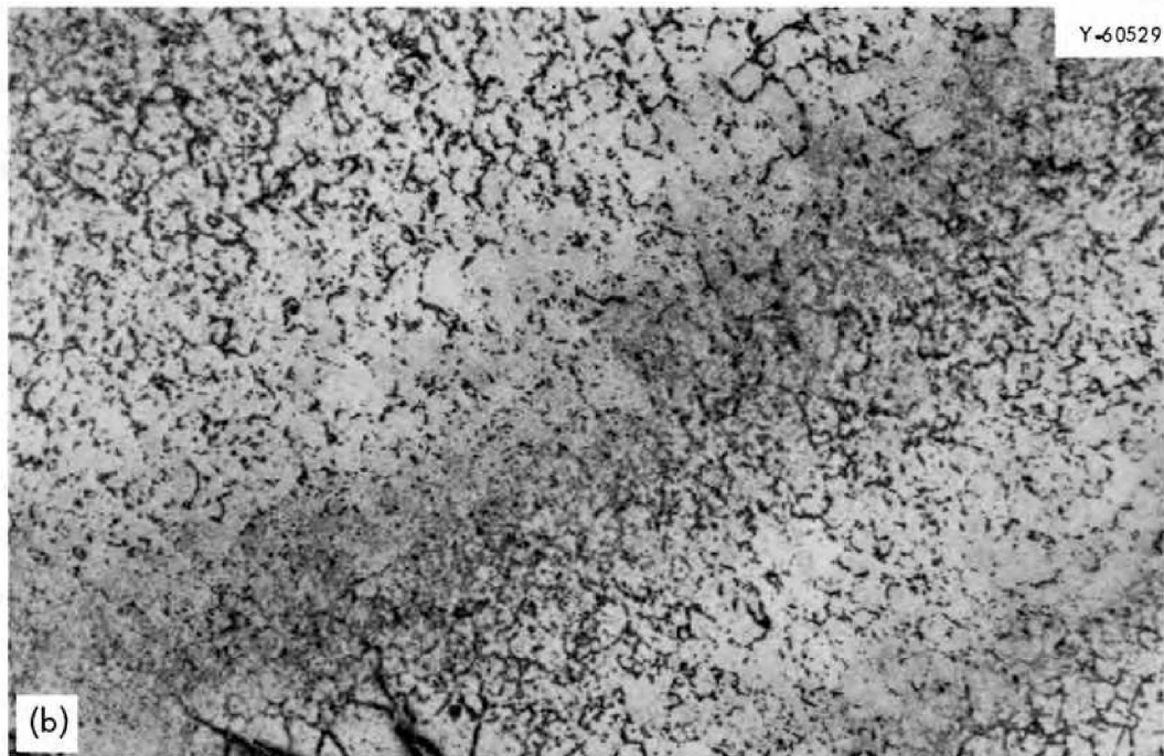
Fig. 10. Autoradiographs of Hastelloy N After a 1-hr Anneal at 1177^{\circ}\text{C} Followed by 100 hr at 649^{\circ}\text{C} . As-polished condition. (a) 16-hr exposure. (b) 72-hr exposure. 250 \times .
