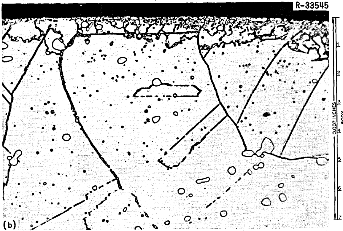
Fig. 30. Cross Section of the Buttonhead of Surveillance Specimen A-16 from Heat 5085 Tested at 25°C. (a) 100 x. (b) 500 x.
