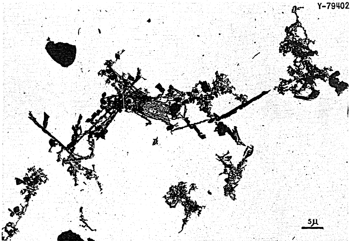
Fig. 35. Extraction Replica From Surveillance Specimen, Heat 5081.
