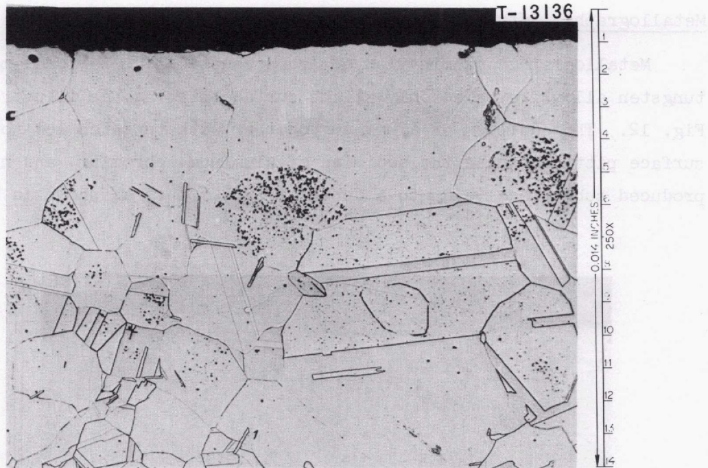
Fig. 11. Appearance of Voids in Nickel-Molybdenum Alloy Containing 3.62 at. % Nb after 1000-hr Exposure to Salt 107. Heat OR 30-21.
