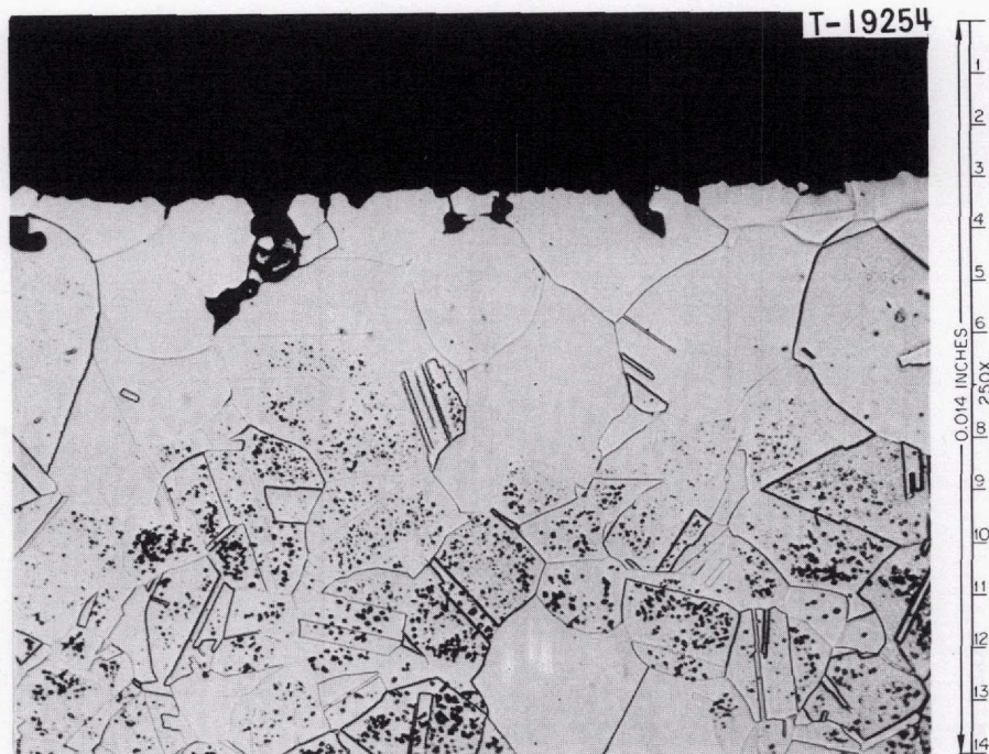
Fig. 10. Attack at Hot-Leg Surface of Ternary Nickel-Molybdenum Alloy Containing 5.11 at. % V. Alloy was exposed to Salt 107 for 1000 hr. Heat OR 30-20.
