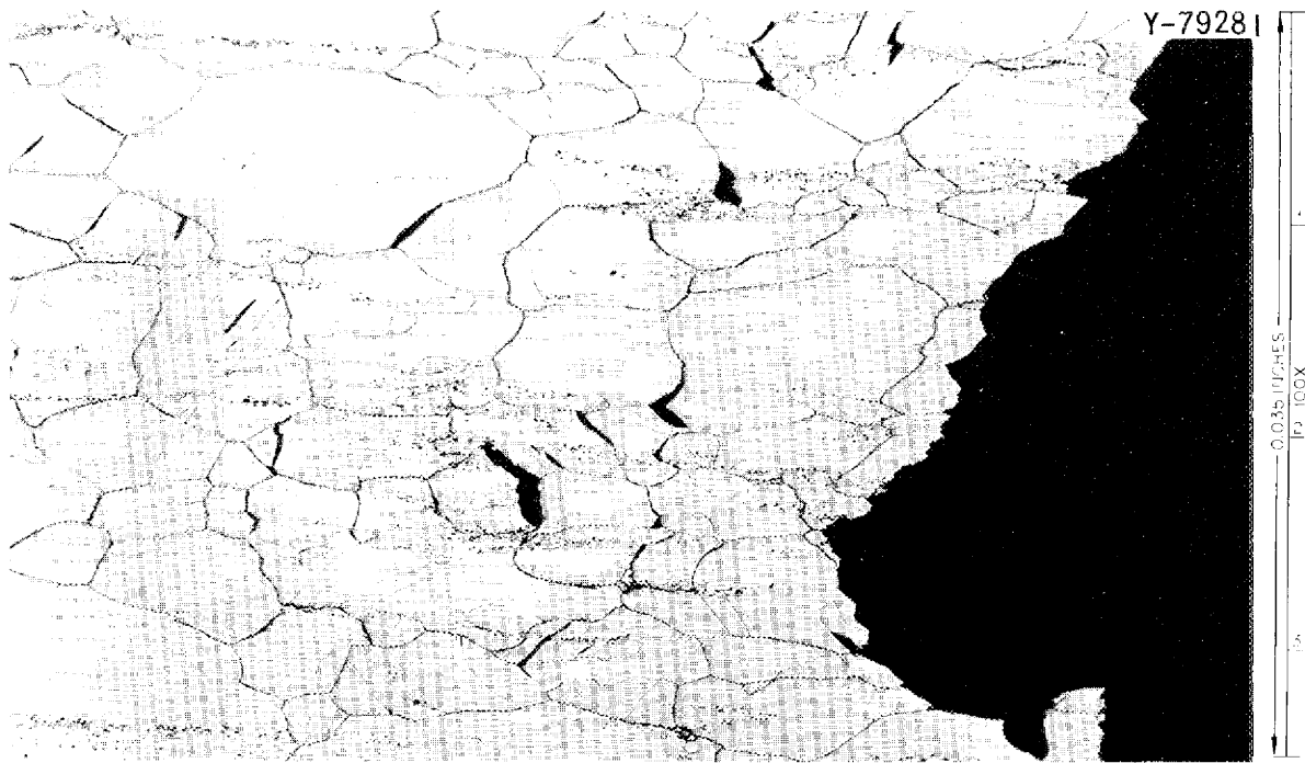
Fig. 21. Photomicrograph of the Fracture of a Specimen from Heat 5911 TH-Anneal 1 Tested at 650°C and at a Strain Rate of 0.002 min -1 . Etchant: glyceria regia.
