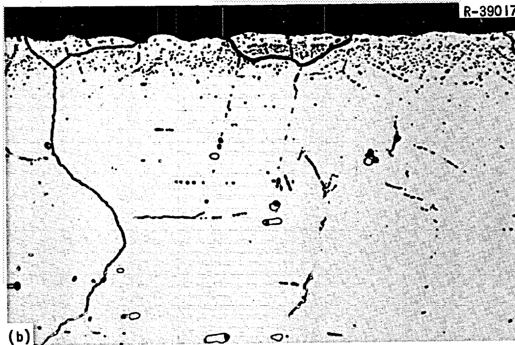
Fig. 7. Photomicrographs of the Edge of the Surveillance Basket Removed from the MSRE after 5500 hr at 650°C. 500X. (a) As polished. Note the grain near the surface that seems almost dislodged. (b) Etchant: Aqua regia. Same area as shown in (a). Note the fine precipitate near the surface.
