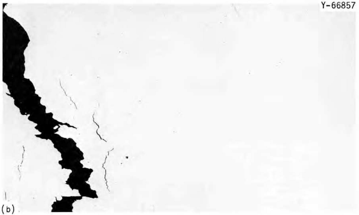
Fig. 19. Photomicrographs of Sample from Weld 1 Tested at 40,000 psi and 1200°F in the As-Welded Condition. Failed in 18.7 hr with 3.1% strain. 100X. (a) Fracture in the weld metal. Etchant: glyceric acid. (b) An unetched photomicrograph of a cracked area away from the fracture.
