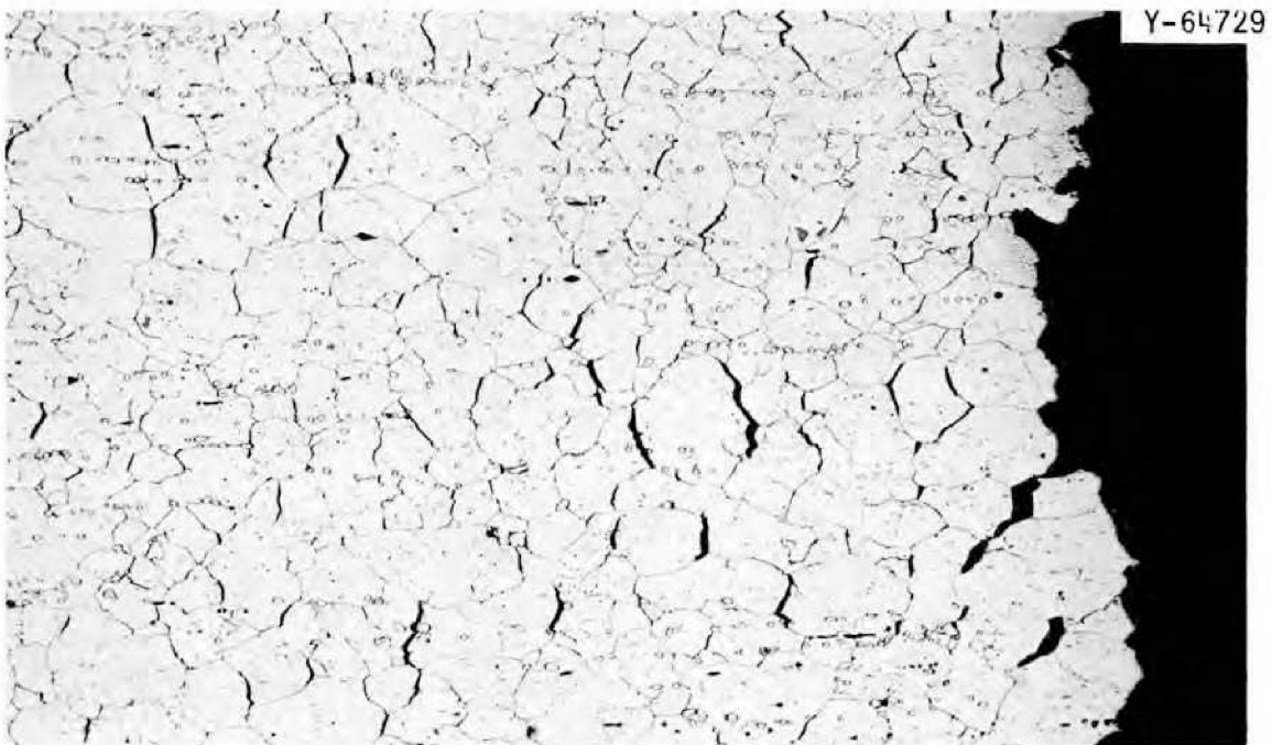
Fig. 18. Photomicrograph of the Fracture of a Hastelloy N (Heat 5065) Sample Tested in Creep at 40,000 psi and 1200°F Following a Pretest Anneal of 1 hr at 2150°F. Failed in 312 hr with 16.6% strain. 100X. Etchant: glyceria regia.
