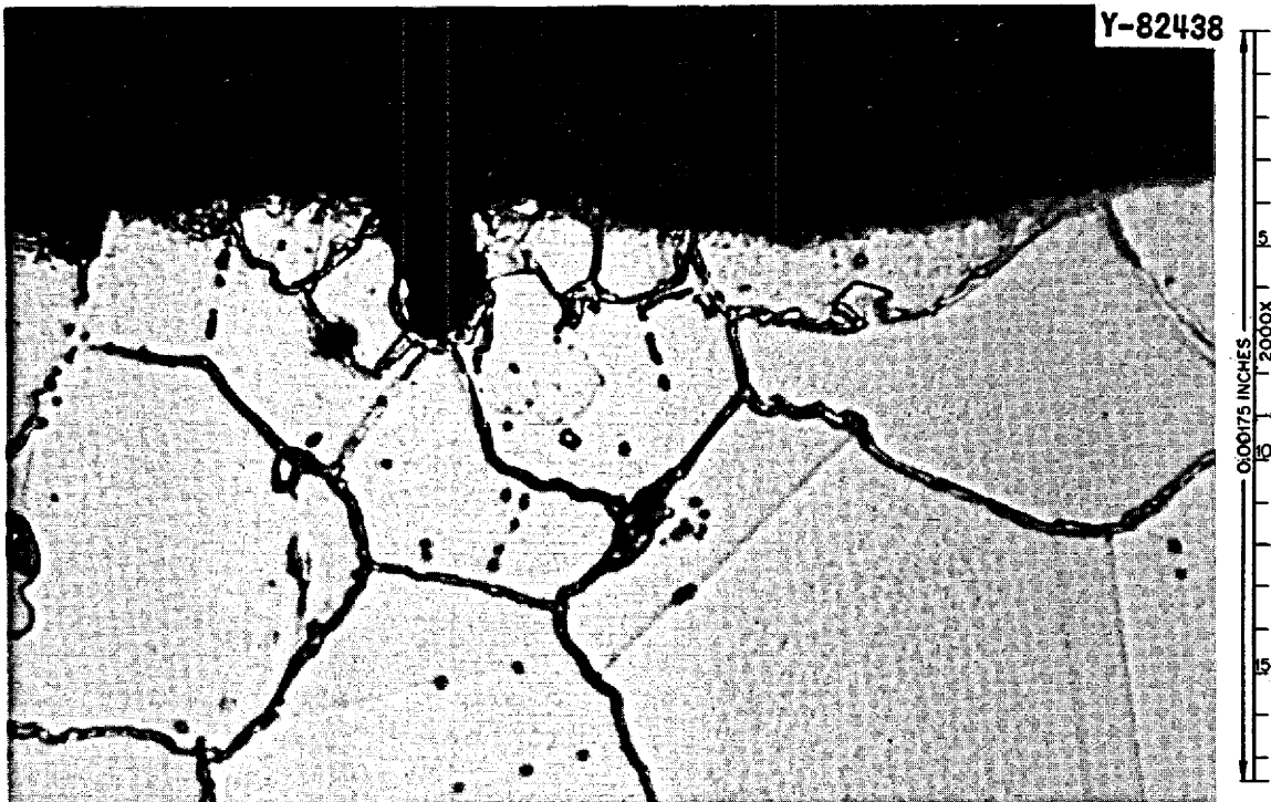
Fig. 7. Hastelloy N Hot-Leg Section NCL-10 (605°C) Shown at Different Magnifications After 8760 hr in Fluoroborate Salt. Etchant: Glyceria Regia.
