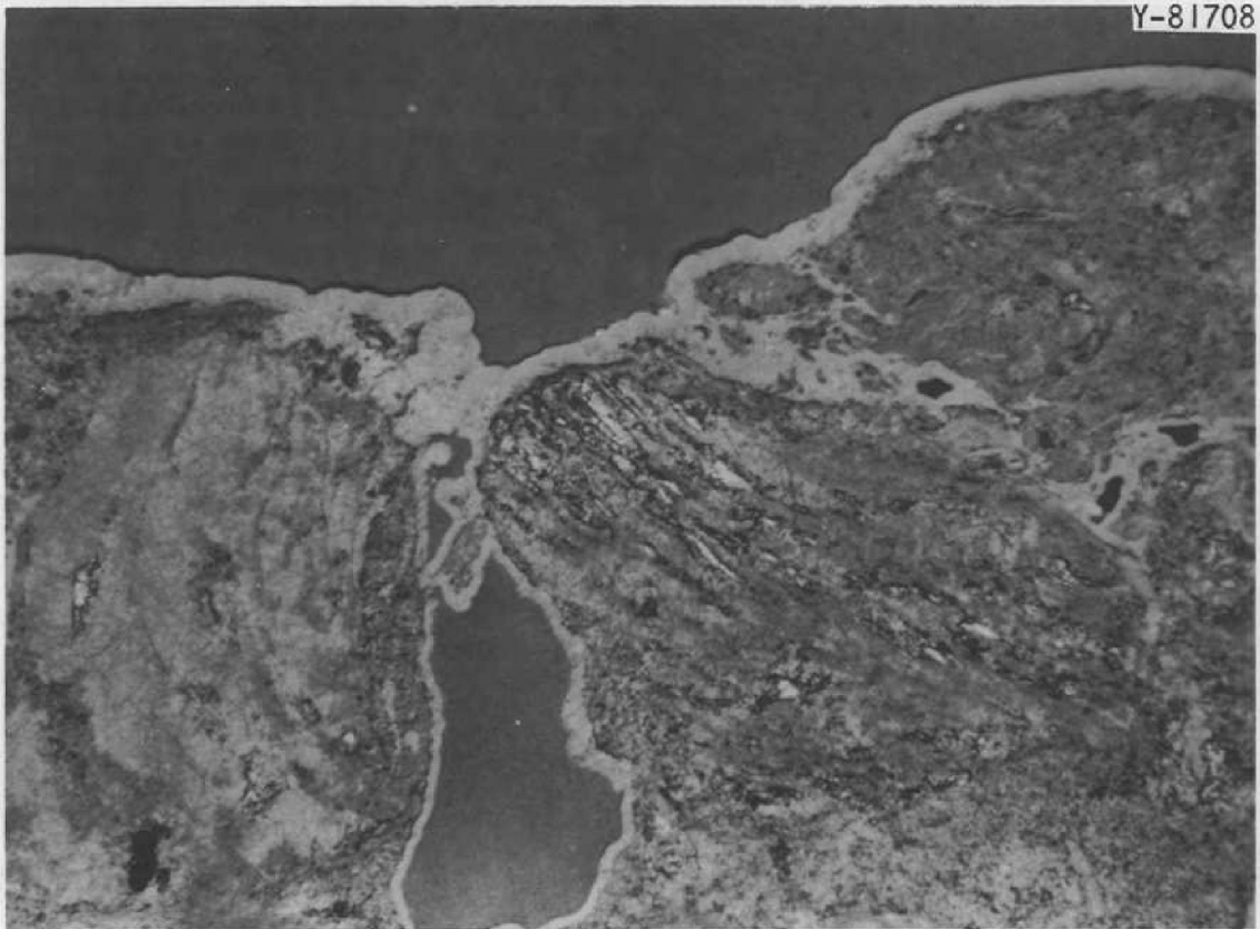
Fig. 10. Photomicrograph of the Edge of Graphite Showing a Pore that has been Partially Coated and then Sealed over with Pyrocarbon.
