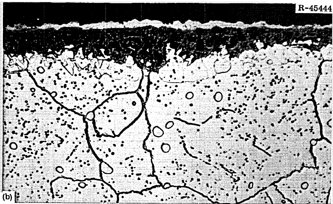
Fig. 3. Photomicrographs of Hastelloy N (Heat 5065) Surveillance Specimens Exposed to the Cell Environment of N_2 + 2 to 5% O_2 for 20,789 hr at 650°C. 500X. (a) Unetched showing surface oxidation. (b) Etched (glyceria regia) showing shallow modification of microstructure due to reaction with cell environment.
