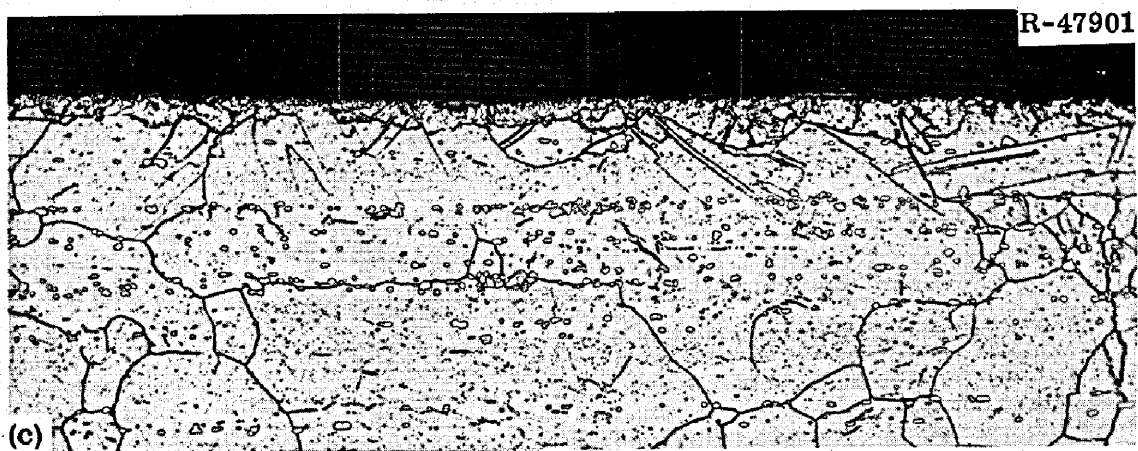
Fig. 37. Photomicrographs of a Hastelloy N (Heat 5085) Sample Tested at 650°C at a Strain Rate of 0.002 min -1 . Sample had been irradiated to a thermal fluence of 2.6 \times 10^{19} neutrons/cm 2 while being exposed to the cell environment at 650°C for 20,789 hr. 100X. (a) Fracture, as polished. (b) Fracture, etched. (c) Edge of stressed portion, etched. Etchant: aqua regia.
