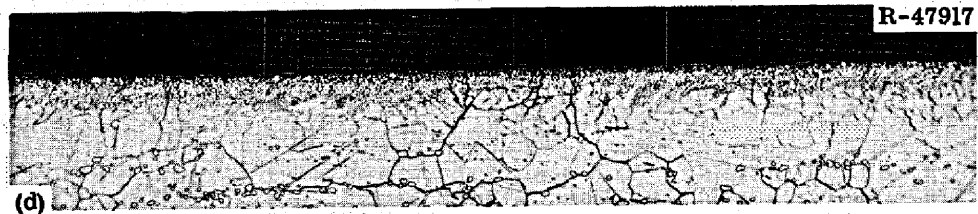
Fig. 43. Photomicrographs of a Hastelloy N (Heat 5085) Sample Exposed to Fluoride Salt in the MSRE for 15,289 hr at 650°C and Then Tested at 650°C and a Strain Rate of 0.002 min -1 . Thermal fluence was 9.4 \times 10^{20} neutrons/cm 2 . (a) Fracture, as polished. 100X. (b) Fracture, as polished. 500X. (c) Fracture, etched. 100X. (d) Edge of stressed portion, etched. 100X. Etchant: aqua regia. Reduced 14.5%.
