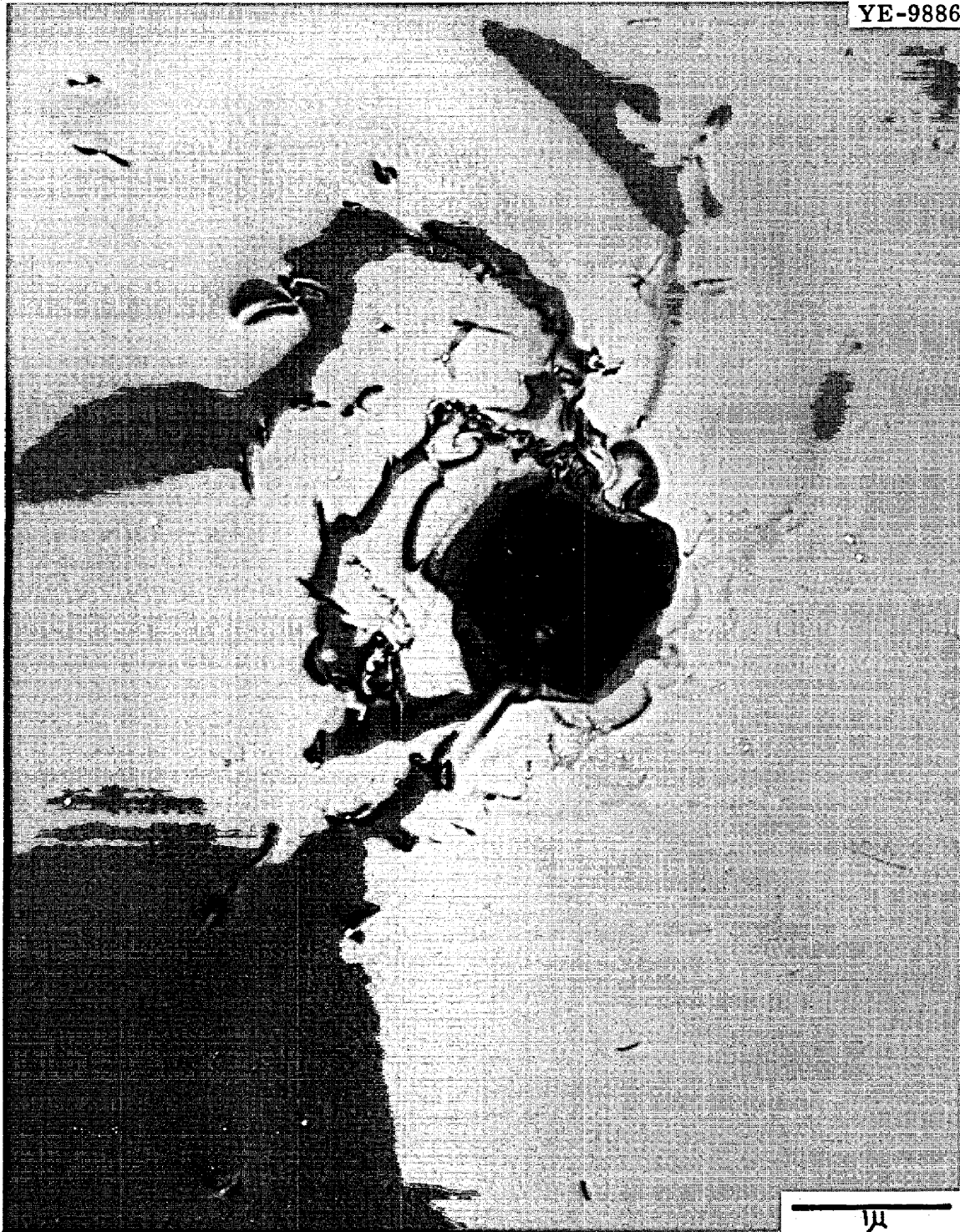
Fig. 8. Transmission Electron Photomicrograph of Hastelloy N (Heat 5085) Exposed to the MSRE Core for 15,289 hr at 650°C. The thermal fluence was 9.4 \times 10^{20} neutrons/cm 2 , enough to transmute most of the 10 B in this material to helium.
