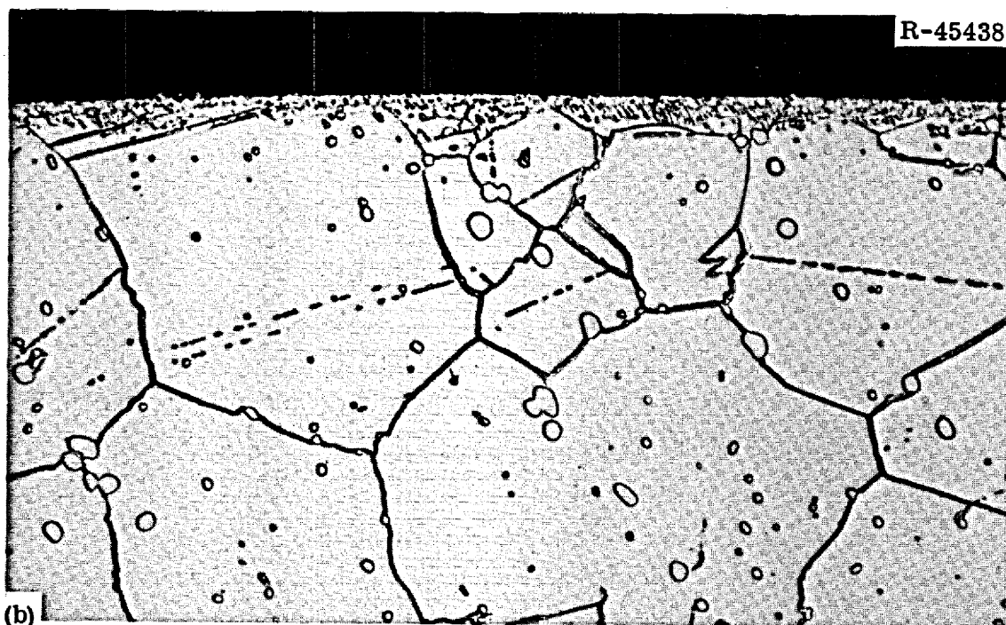
Fig. 4. Photomicrographs of Hastelloy N (Heat 5085) Surveillance Specimens Exposed to Fuel Salt for 15,289 hr at 650°C. 500X. (a) Unetched. (b) Etched (glyceria regia) photomicrographs showing shallow reaction layer near surface.
