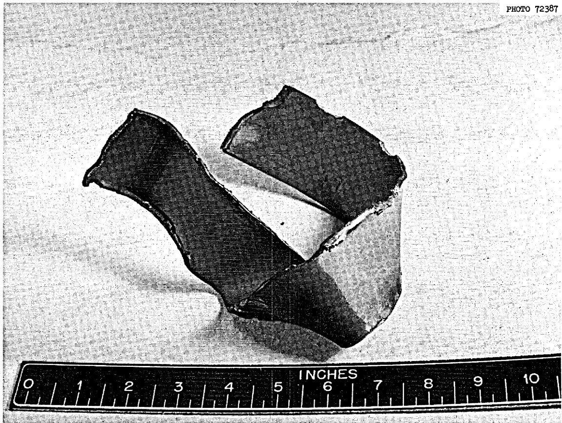
Fig. 12. Part of Flow Straightener After Detachment and Lodging in Impeller Inlet.
