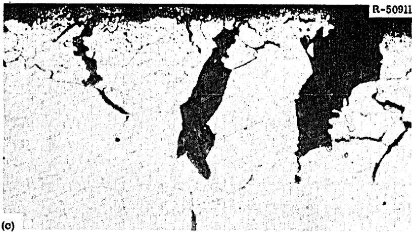
Fig. 48. Photomicrographs of a Hastelloy N (Heat 5065) Sample Tested at 25°C After Being Exposed to the MSRE Core for 22,533 hr at 650°C and Irradiated to a Thermal Fluence of 1.5 \times 10^{21} neutrons/cm 2 . (a) Fracture, etched. 100x. (b) Edge, as polished. 100x. (c) Edge, as polished. 500x. (d) Edge, etched. 100x. Etchant: glyceria regia. Reduced 26%.
