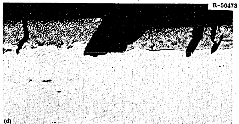
Fig. 60. Photomicrographs of a Modified Hastelloy N (Heat 67-504) Sample Tested at 25°C Following Exposure to the MSRE Cell Environment for 17,033 hr and Irradiation to a Fluence of 2.5 \times 10^{19} neutrons/cm 2 . (a) Fracture, etched. 100X. (b) Edge, as polished. 100X. (c) Edge, etched. 100X. (d) Edge, as polished. 500X. Etchant: glyceria regia. Reduced 27%.
