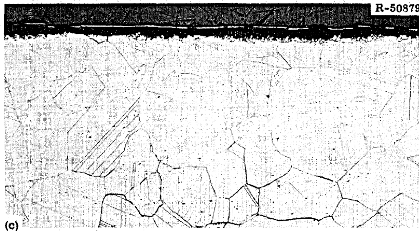
Fig. 61. Photomicrographs of a Modified Hastelloy N (Heat 67-504) Sample Tested at 650°C (Strain Rate, 0.002 min -1 ) Following Exposure to the MSRE Cell Environment for 17,033 hr and Irradiated to a Fluence of 2.5 \times 10^{19} neutrons/cm 2 . (a) Fracture, etched. 100X. (b) Edge, as polished. 100X. (c) Edge, etched. 100X. (d) Edge, as polished. 500X. Etchant: glyceria regia. Reduced 25%.
