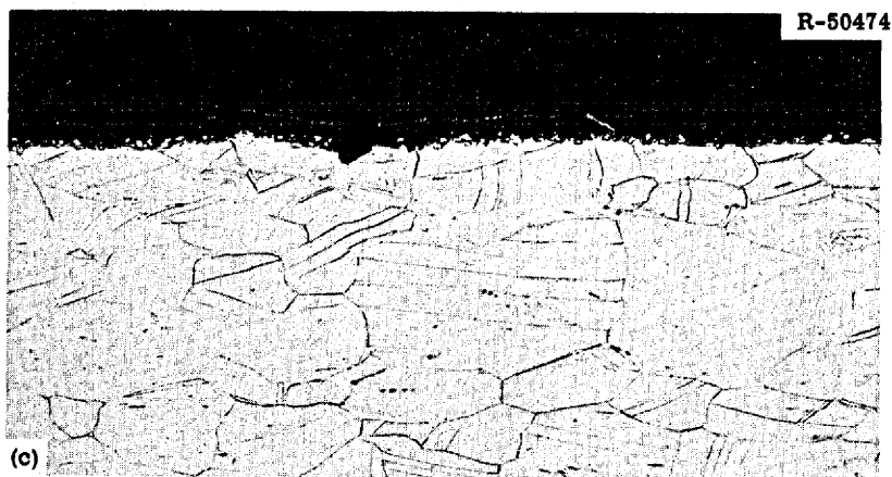
Fig. 60. Photomicrographs of a Modified Hastelloy N (Heat 67-504) Sample Tested at 25°C Following Exposure to the MSRE Cell Environment for 17,033 hr and Irradiation to a Fluence of 2.5 \times 10^{19} neutrons/cm 2 . (a) Fracture, etched. 100X. (b) Edge, as polished. 100X. (c) Edge, etched. 100X. (d) Edge, as polished. 500X. Etchant: glyceria regia. Reduced 27%.
