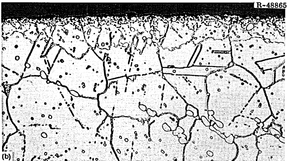
Fig. 4. Typical Photomicrographs of Hastelloy N (Heat 5085) Exposed to the MSRE Core for 22,533 hr at 650°C. (a) As polished. (b) Etchant: glyceric acid. 500X.
