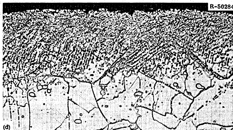
Fig. 5. Typical Photomicrographs of a Hastelloy N (Heat 5085) Sample Exposed to the MSRE Core for 22,533 hr at 650°C. The sample was bent in a vise. (a) As polished, tension side. (b) As polished, tension side. (c) Etched, tension side. (d) Etched, compression side. Etchant: aqua regia. 500X. Reduced 27%.
