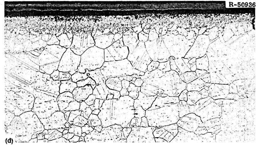
Fig. 45. Photomicrographs of a Hastelloy N (Heat 5085) Sample Tested at 650°C After Being Exposed to the Core of the MSRE for 22,533 hr at 650°C and Irradiated to a Thermal Fluence of 1.5 \times 10^{21} neutrons/cm 2 . (a) Fracture, etched. 100X. (b) Edge, as polished. 100X. (c) Edge, as polished. 500X. (d) Edge, etched. 100X. Etchant: glyceria regia. Reduced 27%.
