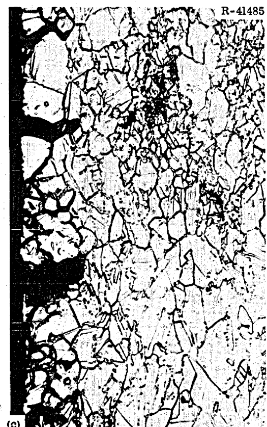
Fig. 72. Photomicrographs of a Zirconium-Modified Hastelloy N Surveillance Sample (Heat 21554) Tested at 25°C at a Strain Rate of 0.05 min -1 . Exposed in the Molten Salt Reactor Experiment core for 5500 hr at 650°C to a thermal-neutron fluence of 4.1 \times 10^{20} neutrons/cm 2 . (a) Fracture, 100X; (b) edge of sample about 1/2 in. from fracture, 100X; and (c) edge of sample showing edge cracking, 500X. Etchant: aqua regia. Reduced 24%.
