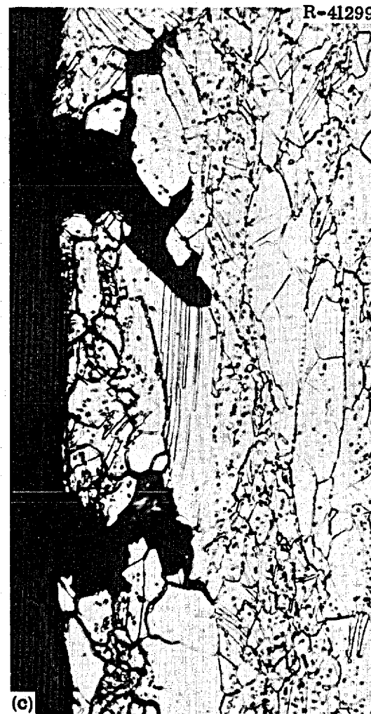
Fig. 32. Photomicrographs of a Titanium-Modified Hastelloy N Surveillance Sample (Heat 21545) Tested at 25°C at a Strain Rate of 0.05 min -1 . Exposed in the MSRE core for 5500 hr at 650°C to a thermal fluence of 4.1 \times 10^{20} neutrons/cm 2 . (a) Fracture, 100X; (b) edge of sample about 1/2 in. from fracture, 100X; (c) edge of sample showing edge cracking, 500X. Etchant: aqua regia. Reduced 8%.
