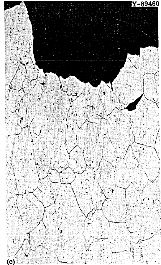
Fig. 67. Photomicrographs of Alloy 21555 (0.05% Zr) Creep Tested at 32,400 psi and 650°C. (a) Fracture of sample annealed for 100 hr at 871°C and 1000 hr at 650°C before test; (b) fracture of sample annealed 1 hr at 1177°C before test; and (c) fracture of sample annealed 1 hr at 1177°C and 1000 hr at 650°C. 100X. Etchant: glyceria regia. Reduced 21%.
