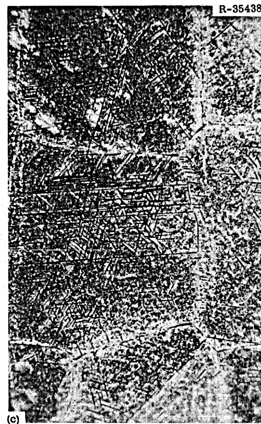
Fig. 70. Photomicrographs of Alloy 110 (0.53% Zr) Annealed 1 hr at 1177°C, Irradiated at 650°C for 1000 hr to a Thermal-Neutron Fluence of 2.5 \times 10^{20} neutrons/cm 2 , and Creep Tested at 650°C. Stressed at 32,400 psi for 675 hr (0.97% Strain) and 40,000 psi for 430 hr (5.9% Strain). (a) Fracture, 100X; (b) edge of gage length, 100X; and (c) typical, 1000X. Etchant: glyceria regia. Reduced 24%.
