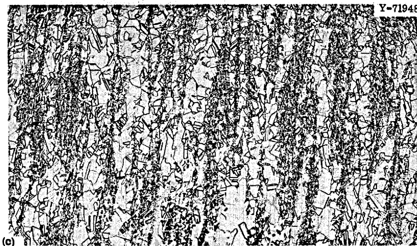
Fig. 4. Photomicrographs of Heat 21545, which contained 0.49% Ti. (a) Annealed 1 hr at 1177°C, 100x; (b) precipitate after anneal of 1 hr at 1177°C, 1000x; (c) and (d) annealed 100 hr at 871°C, 100 and 500x. Samples (a), (c), and (d) etched with glyceric regia. Sample (b) etched with hydrochloric, nitric, and lactic acids. Reduced 28%.
