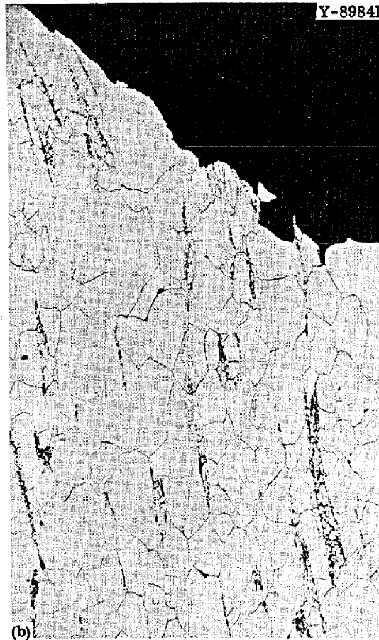
Fig. 67. Photomicrographs of Alloy 21555 (0.05% Zr) Creep Tested at 32,400 psi and 650°C. (a) Fracture of sample annealed for 100 hr at 871°C and 1000 hr at 650°C before test; (b) fracture of sample annealed 1 hr at 1177°C before test; and (c) fracture of sample annealed 1 hr at 1177°C and 1000 hr at 650°C. 100X. Etchant: glyceria regia. Reduced 21%.
