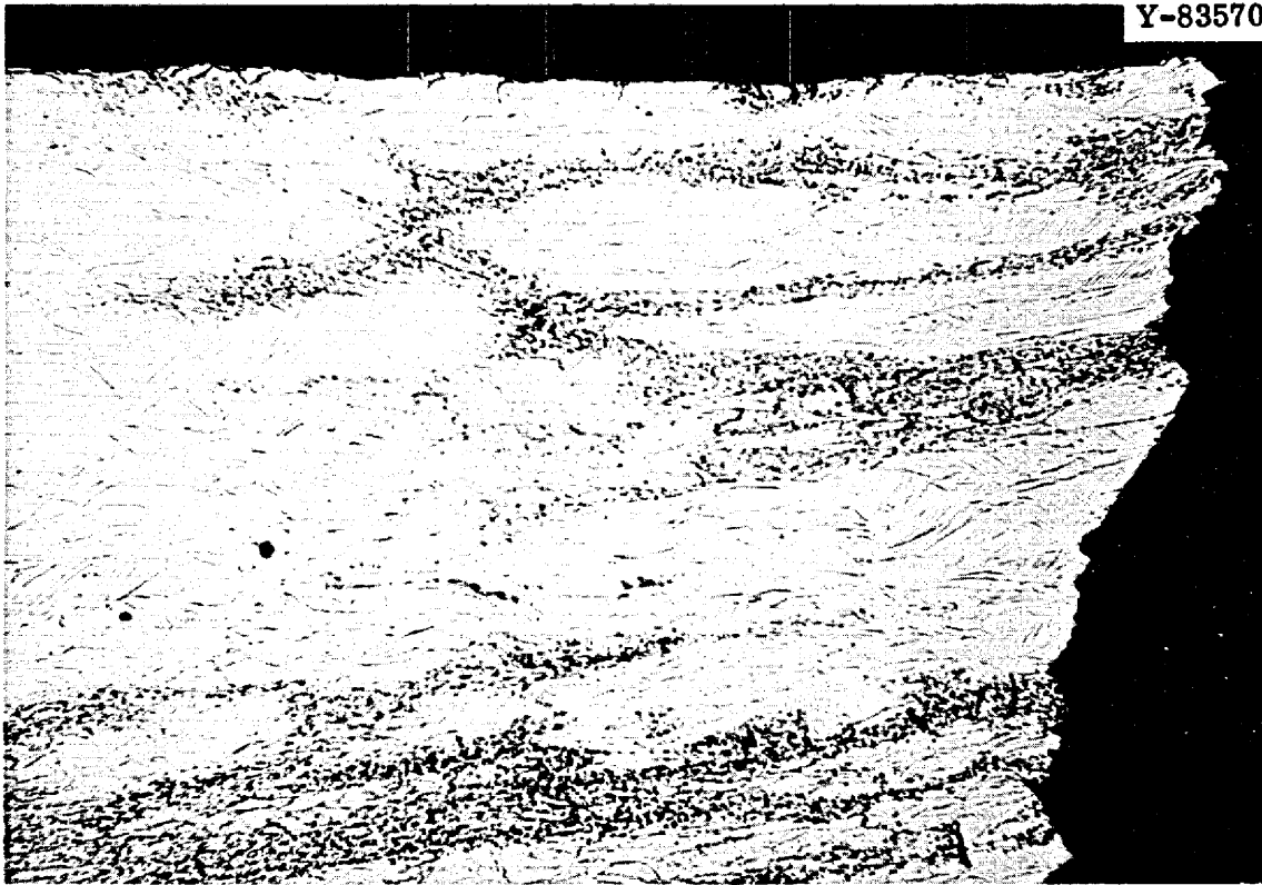
Fig. 33. Photomicrograph of the Fracture of a Titanium-Modified Hastelloy N Surveillance Sample (Heat 21545) Tested at 25°C at a Strain Rate of 0.05 min -1 . Exposed to a static fluoride salt for 5500 hr at 650°C before testing. Note the shear fracture and the absence of edge cracking. 100X. Etchant: glyceria regia.
