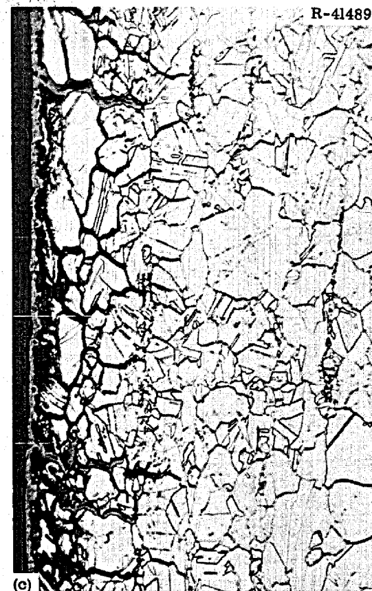
Fig. 74. Photomicrographs of a Zirconium-Modified Hastelloy N Surveillance Sample (Heat 21554) Tested at 650°C at a Strain Rate of 0.002 min -1 . Exposed in the Molten Salt Reactor Experiment core for 5500 hr at 650°C to a thermal fluence of 4.1 \times 10^{20} neutrons/cm 2 . (a) Fracture, 100x; (b) edge of sample about 1/2 in. from fracture, 100x; and (c) edge of sample showing edge cracking. Oxide formed during the tensile test. 500x. Etchant: aqua regia. Reduced 22%.
