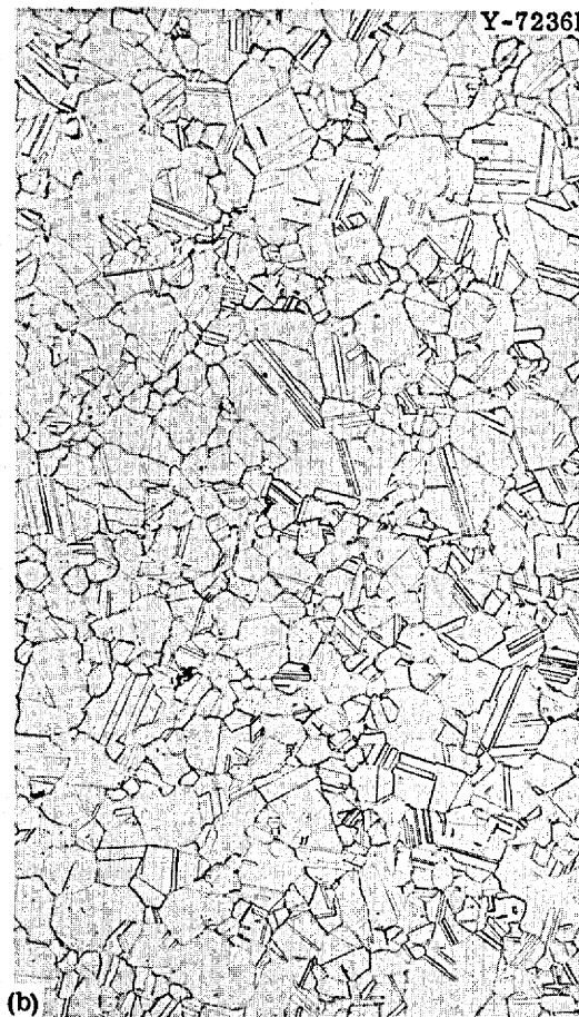
Fig. 76. Photomicrographs of Alloys Modified with Hafnium Annealed 1 hr at 1177°C. (a) Alloy 153 (0.06% Hf); (b) alloy 154 (0.10% Hf) and (c) alloy 155 (0.13% Hf). 100x. Etchant: glyceria regia. Reduced 18%.
