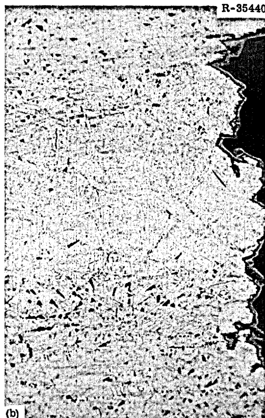
Fig. 71. Photomicrographs of Alloy 112 (1.18% Zr) Annealed 1 hr at 1177°C, Irradiated at 650°C for 1000 hr to a Thermal-Neutron Fluence of 2.5 \times 10^{20} neutrons/cm 2 , and Creep Tested at 650°C. Stressed at 32,400 psi for 677 hr (5.8% Strain) and 40,000 psi for 47 hr (3.9% Strain). (a) Fracture, 100x; (b) fracture, 500x; and (c) typical, 1000x. Etchant: glyceria regia. Reduced 24%.
