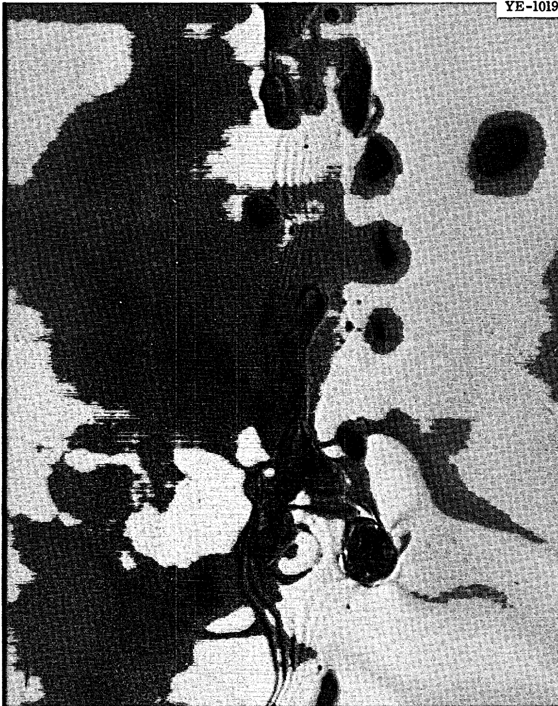
Fig. 109. Transmission Electron Photomicrograph of Alloy 21546 after Irradiation at 766°C for about 1100 hr to a Thermal-Neutron Fluence of 2.4 \times 10^{20} neutrons/cm 2 . 50,000X.
