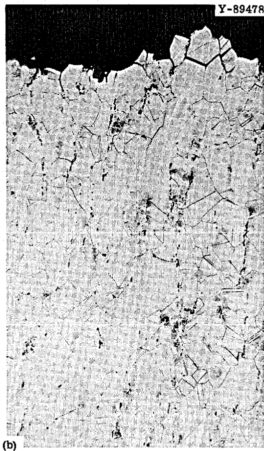
Fig. 68. Photomicrographs of Alloy 21554 (0.35% Zr) Creep Tested at 650°C. (a) Fracture of sample annealed 100 hr at 871°C and 1000 hr at 650°C before test; (b) fracture of a sample annealed 1 hr at 1177°C before test; and (c) fracture of a sample annealed 1 hr at 1177°C and 1000 hr at 650°C before test. 100X. Etchant: glyceria regia. Reduced 21%.
