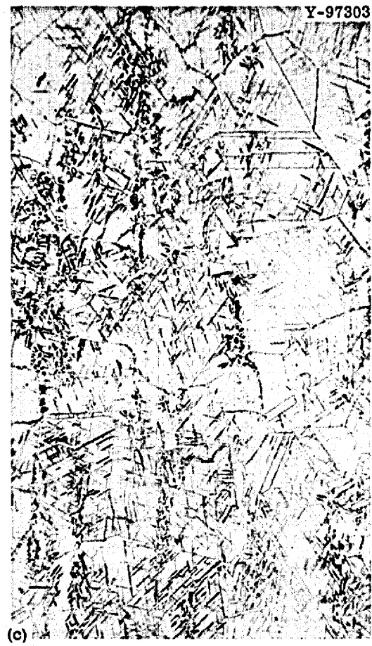
Fig. 66. Photomicrographs of Alloy 112 (1.18% Zr) Annealed 1 hr at 1177°C and Tested at 650°C and 47,000 psi. (a) Fracture, 100X; (b) typical, 100X, and (c) typical, 500X. Etchant: glyceria regia. Reduced 20%.
