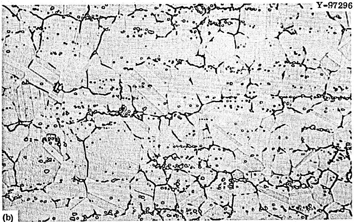
Fig. 27. Photomicrographs of Alloy 107 (1.04% Ti) after Annealing 1 hr at 1177°C and Testing at 650°C and 40,000 psi. (a) Fracture, 100X; (b) typical, 500X. Etchant, glyceric regia.
