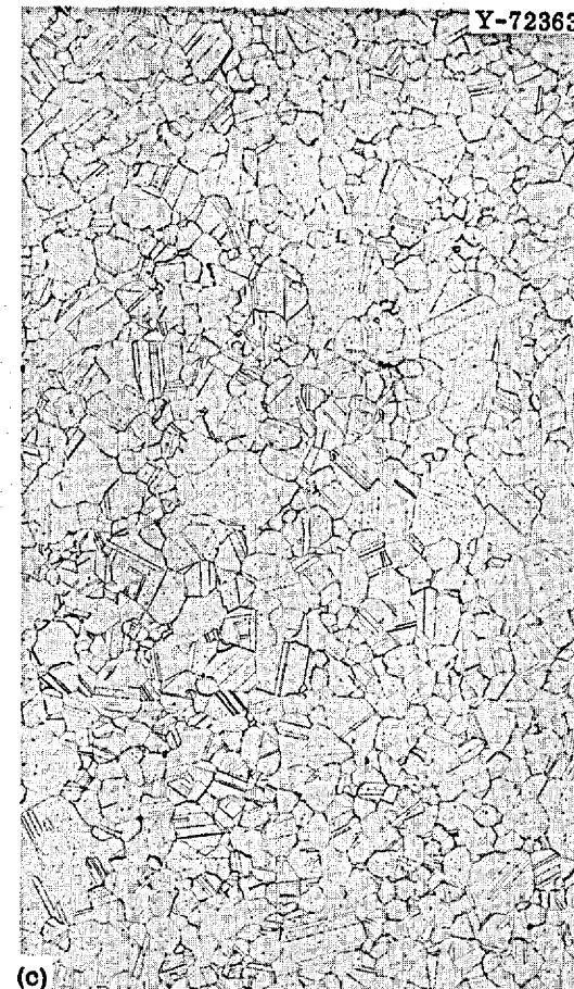
Fig. 76. Photomicrographs of Alloys Modified with Hafnium Annealed 1 hr at 1177°C. (a) Alloy 153 (0.06% Hf); (b) alloy 154 (0.10% Hf) and (c) alloy 155 (0.13% Hf). 100x. Etchant: glyceria regia. Reduced 18%.
