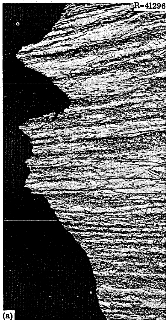
Fig. 32. Photomicrographs of a Titanium-Modified Hastelloy N Surveillance Sample (Heat 21545) Tested at 25°C at a Strain Rate of 0.05 min -1 . Exposed in the MSRE core for 5500 hr at 650°C to a thermal fluence of 4.1 \times 10^{20} neutrons/cm 2 . (a) Fracture, 100X; (b) edge of sample about 1/2 in. from fracture, 100X; (c) edge of sample showing edge cracking, 500X. Etchant: aqua regia. Reduced 8%.
