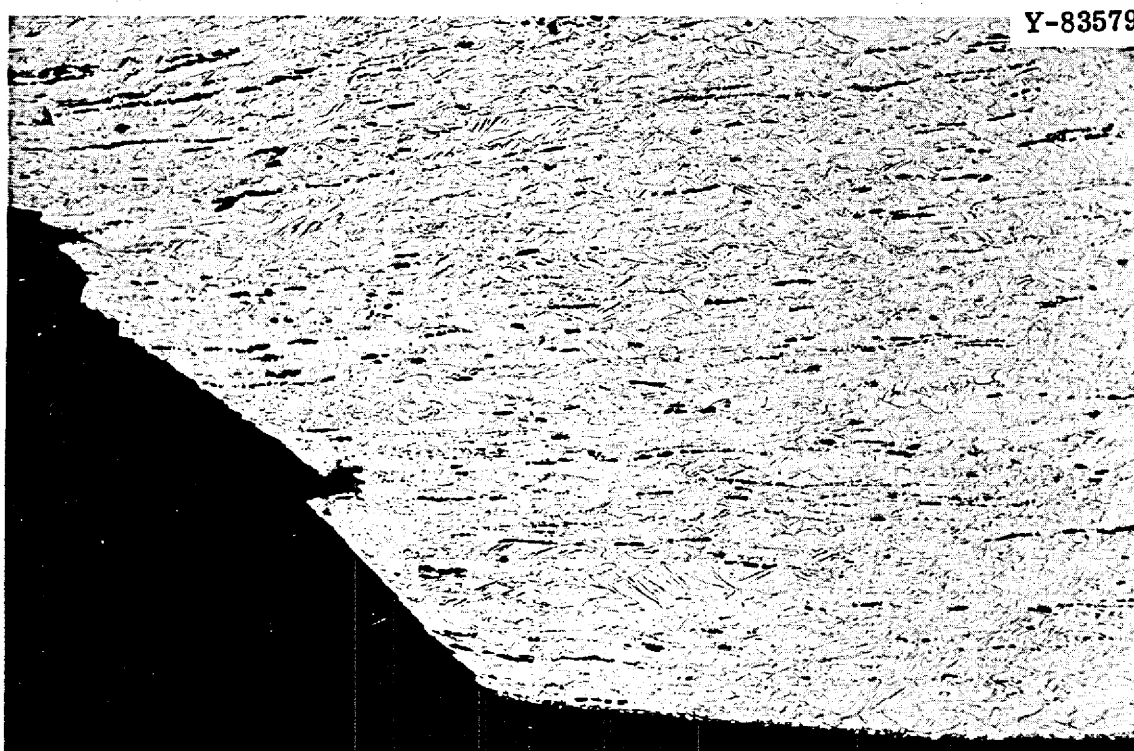
Fig. 73. Photomicrograph of the Fracture of a Zirconium-Modified Hastelloy N Sample (Heat 21554) Tested at 25°C at a Strain Rate of 0.05 min -1 . Exposed to a static fluoride salt for 5500 hr at 650°C before testing. Note the shear fracture and the absence of edge cracking. 100x. Etchant: glyceria regia.
