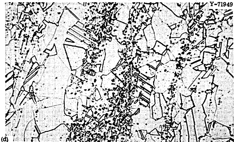
Fig. 4. Photomicrographs of Heat 21545, which contained 0.49% Ti. (a) Annealed 1 hr at 1177°C, 100x; (b) precipitate after anneal of 1 hr at 1177°C, 1000x; (c) and (d) annealed 100 hr at 871°C, 100 and 500x. Samples (a), (c), and (d) etched with glyceric regia. Sample (b) etched with hydrochloric, nitric, and lactic acids. Reduced 28%.
