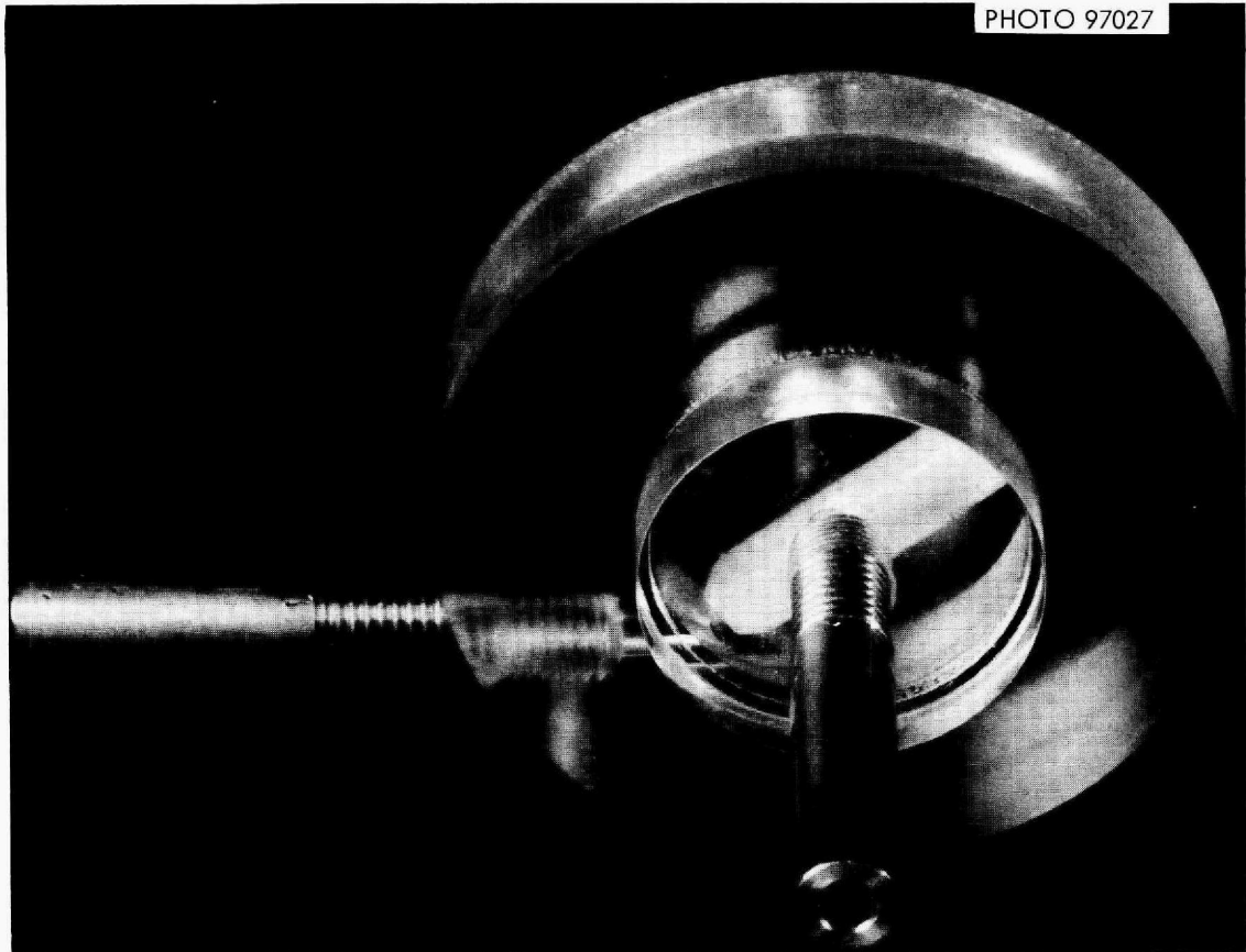
Fig. 3. Magnetically Driven Centrifugal Pump Used for Circulating Solution from Column Through Photocell.
