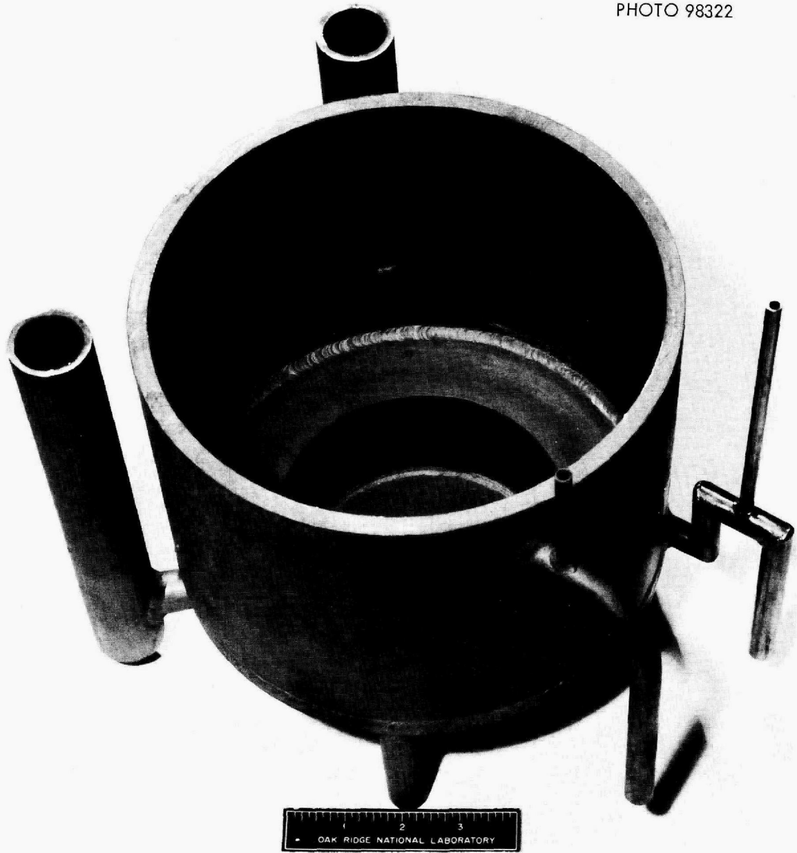
Fig. 58. Cell Vessel for Flowing Salt and Bismuth Streams Through the Bismuth Cathode Pool and the Electrolyte Pool.
