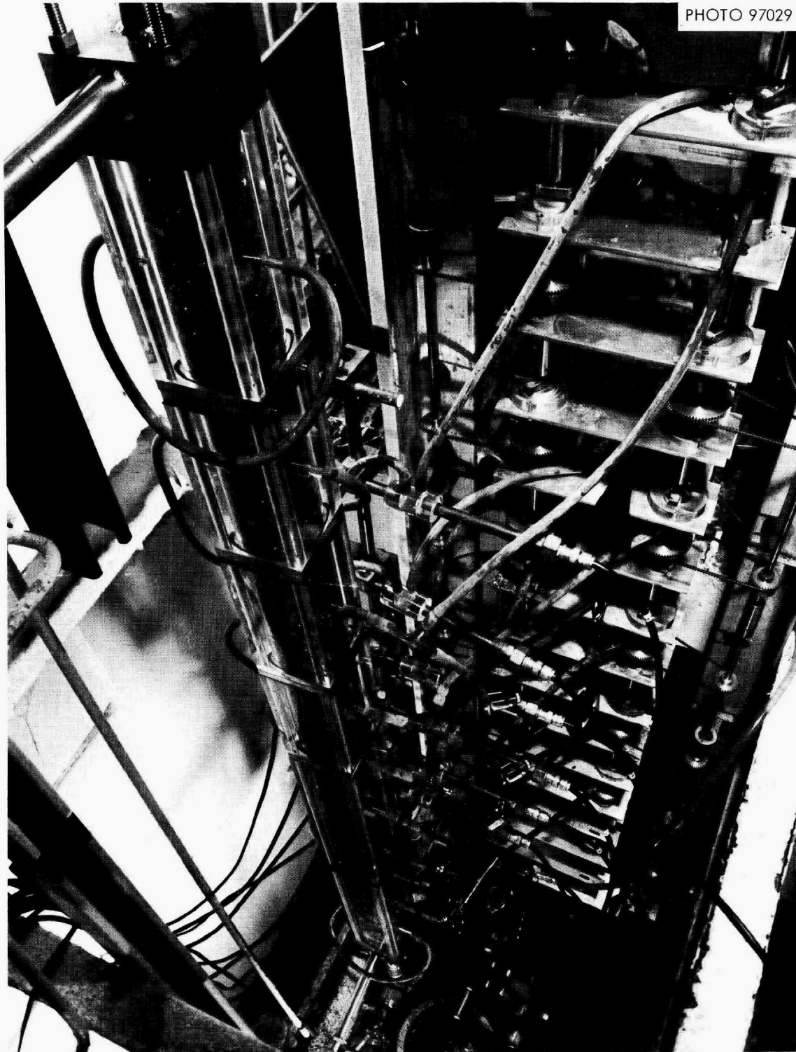
Fig. 2. Equipment Used for Study of Axial Dispersion in a Packed Column During Countercurrent Flow of Mercury and Water.
