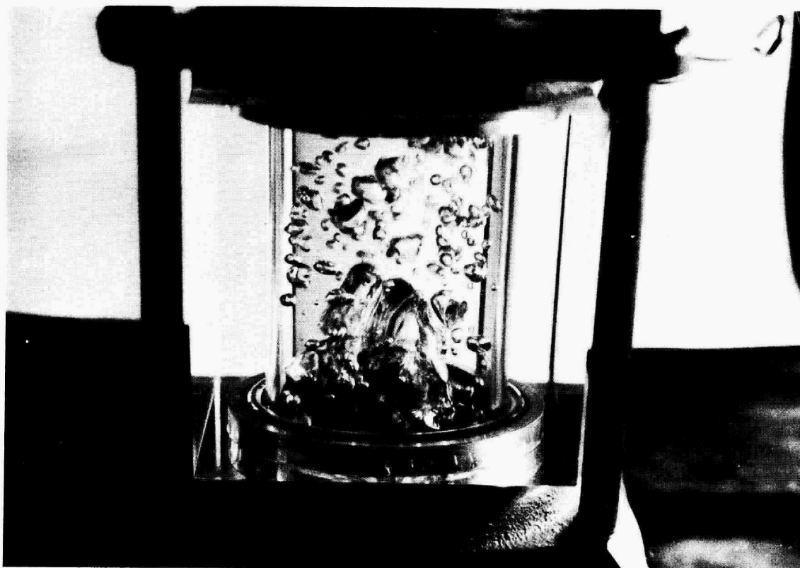
Fig. 45. Air Bubble Distribution During Countercurrent Flow of Air and Water in a 2-in.-diam Open Bubble Column. Gas flow rate, 58 \text{ cm}^3/\text{sec} ; water superficial velocity, 0.130 \text{ cm}/\text{sec} .
