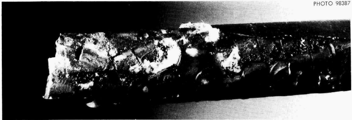
Fig. 14. Section of 0.082-in.-ID Column Showing Dendritic Iron Deposit (Upper Photograph). The lower half of the column was potted in epoxy resin, and the steel pipe was stripped away.
