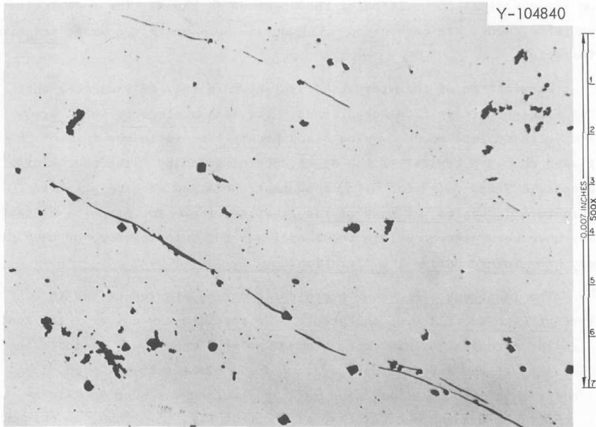
Fig. 62. Photomicrograph Showing Microstructure of Steel from Salt Feed-and-Catch Tank in the As-Polished Condition After Operation at 600 to 700°C for 16,000 hr. Magnification, 500X.
