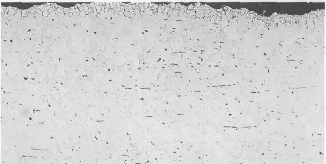
Fig. 60. Photomicrographs of the Inner Surface of the Salt Feed-and-Catch Tank in the (a) As Polished and (b) Etched Condition After Exposure to Salt at 600 to 700°C for 16,000 hr. Magnification, 100X. Etchant, 2% Nital.
