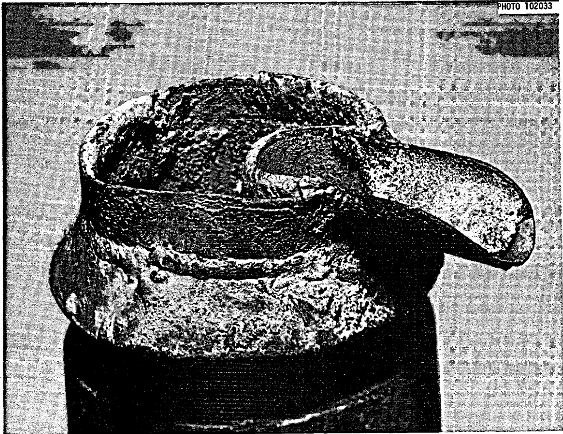
Fig. 8. View of Upper Section of the Li-Bi Container Showing Metallic Deposit on the Rim After Completion of Metal Transfer Experiment MTE-2.
