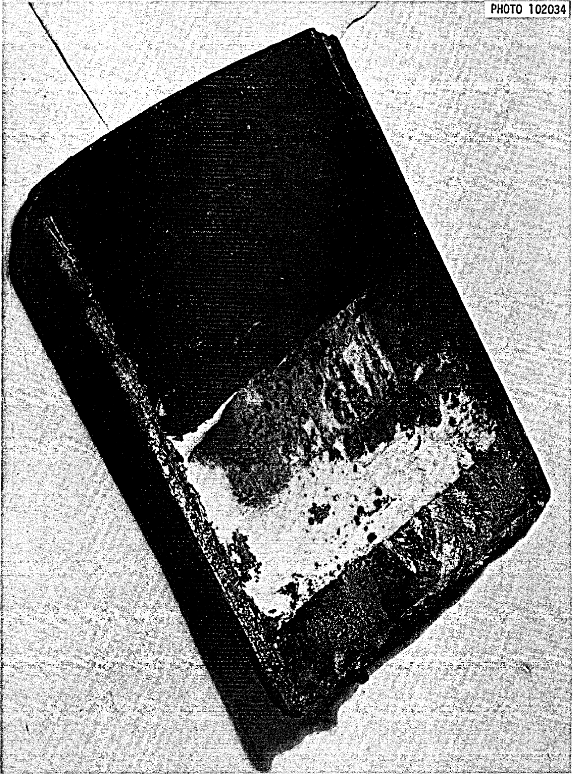
Fig. 6. Salt and Bismuth Phases from the Fluoride Salt Compartment on Completion of Metal Transfer Experiment MTE-2.
