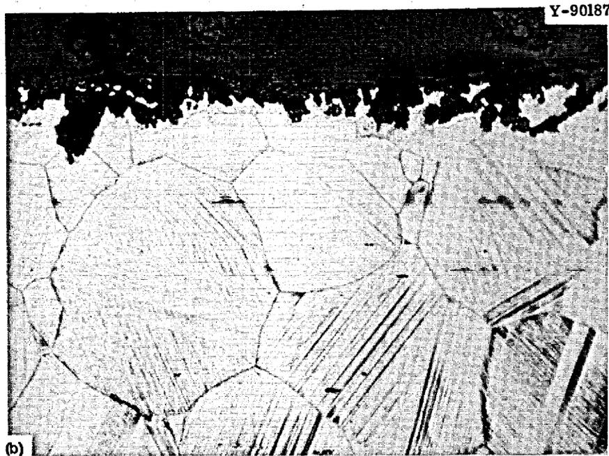
Fig. 4. Microstructure of Haynes Alloy No. 25 Exposed to  $\text{BF}_3$  Gas at  $604^\circ\text{C}$  in NCL-13 for 3660 hr. 500X. (a) Area of greatest attack. (b) Remainder of sample. Etchant is hydrochloric acid and hydrogen peroxide.
