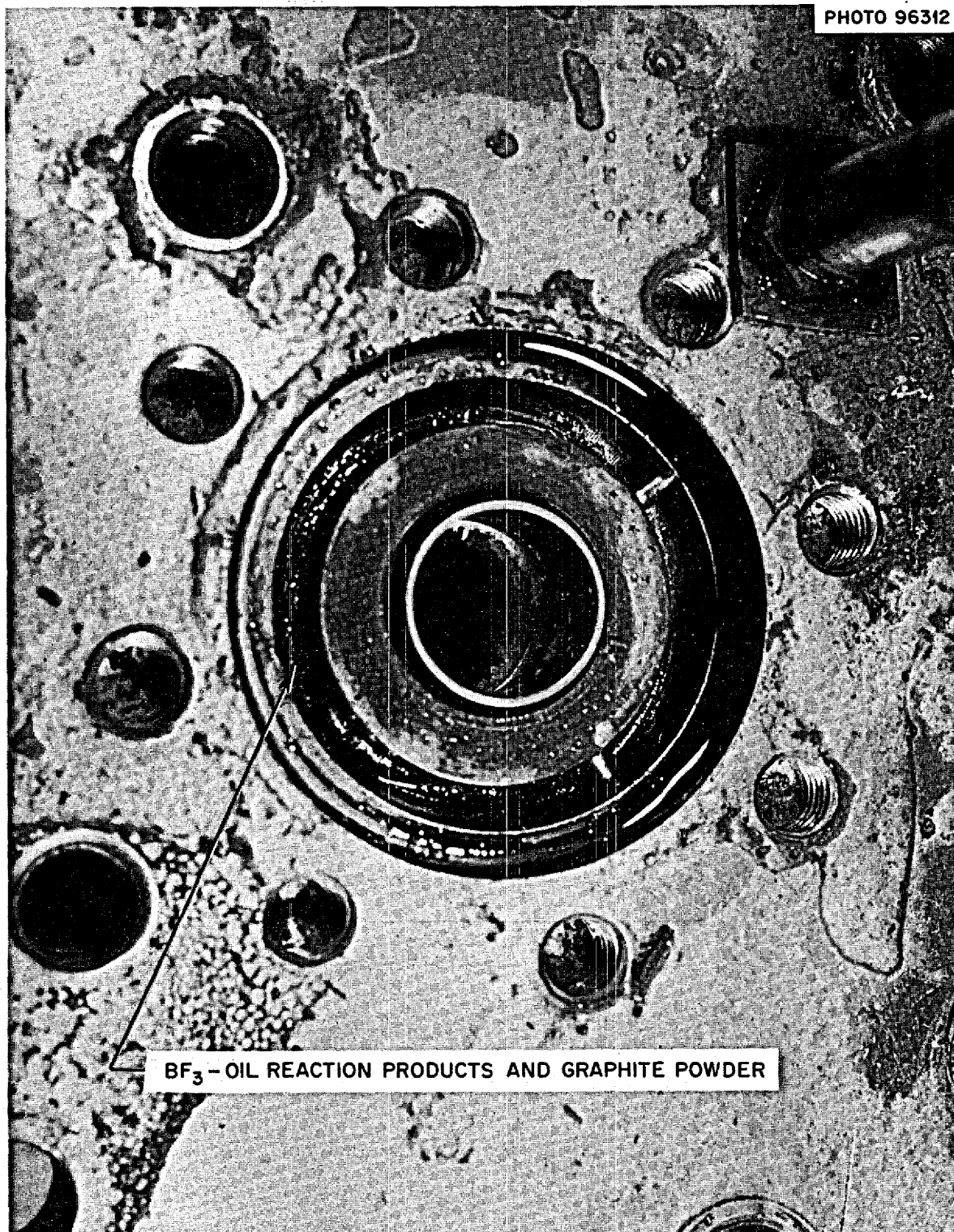
Fig. 18. Typical appearance of the seal oil catch basin of the salt pump after 2000 hr operation (model LFB pump).
