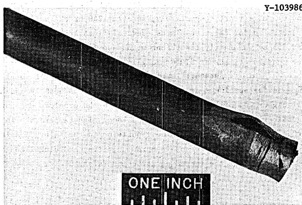
Fig. 32. Tube Ruptured During Salt Melting after Run 6, Loop MSR-FCL-1.
