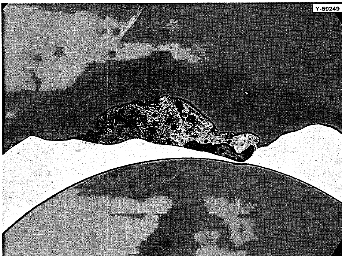
Fig. 7. Cross section of oxidized region adjacent to hole in failed section of loop. As polished, about 14X.
