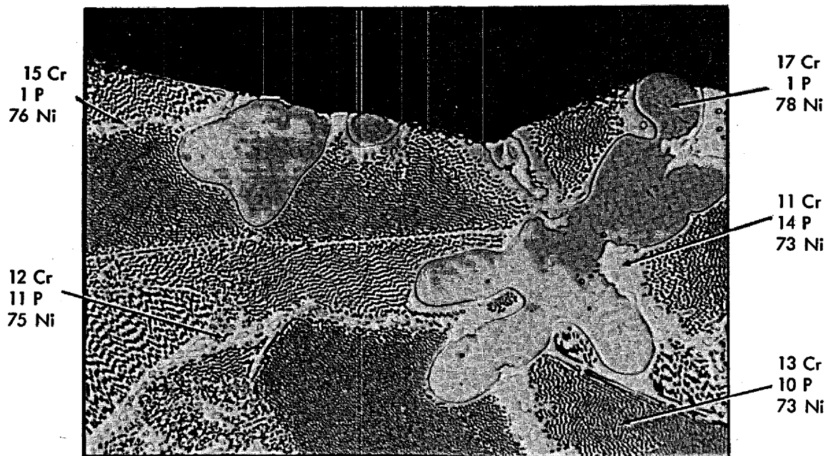
Fig. 5. Microstructural analysis of BNi-7 (Ni-13% Cr-10% P) braze fillet. As-polished. 500X. Top - as-brazed; bottom - exposed to \text{NaBF}_4 -8 mole % NaF for 4987 hr at 610°C. Reduced 19%.
