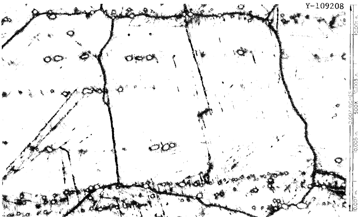
Fig. 17. Typical Photomicrograph of Haynes Alloy No. 25 Annealed 1 hr at 1150°C and Aged 4843 hr at 700°C. Impact energy at 25°C was 5 ft-lb. Etchant: glyceria regia.
