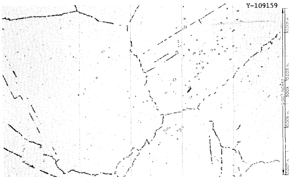
Fig. 13. Typical Photomicrograph of Hastelloy N Annealed 1 hr at 1150°C and Aged 4000 hr at 800°C. Impact energy was 40 ft-lb. Etchant: glyceria regia.
