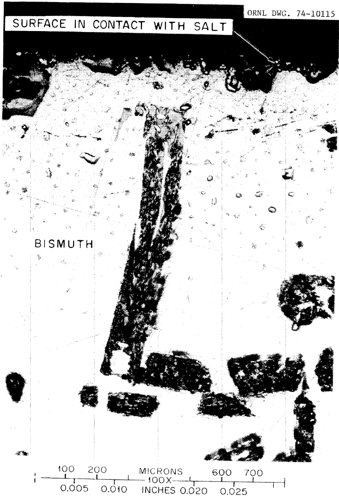
Fig. 10. Photomicrograph of Li-Bi phase from the stripper vessel at the LiCl interface in experiment MTE-3. As polished. 100X.
