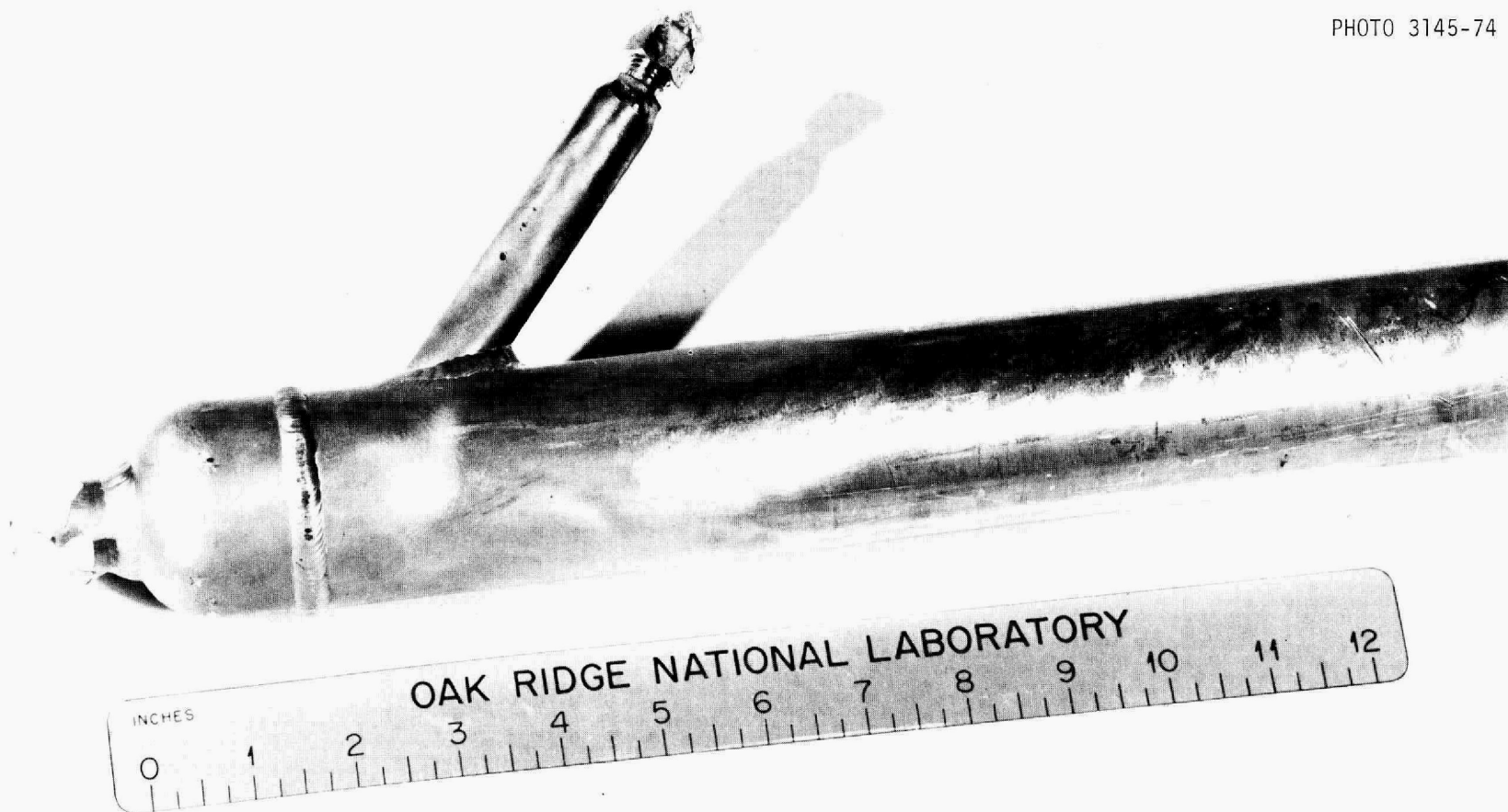
Fig. 15. View near bottom of H_2 reduction column for FREE.
