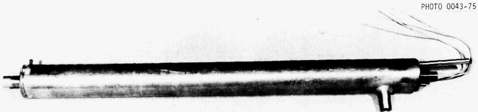
Fig. 7. Heat flowmeter used in autoresistance heating test AHT-4.
