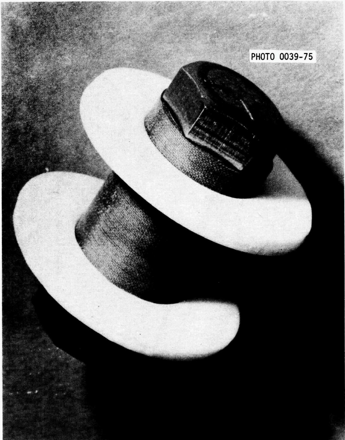
Fig. 2. Insulated bolts used with electrical isolation flanges.
