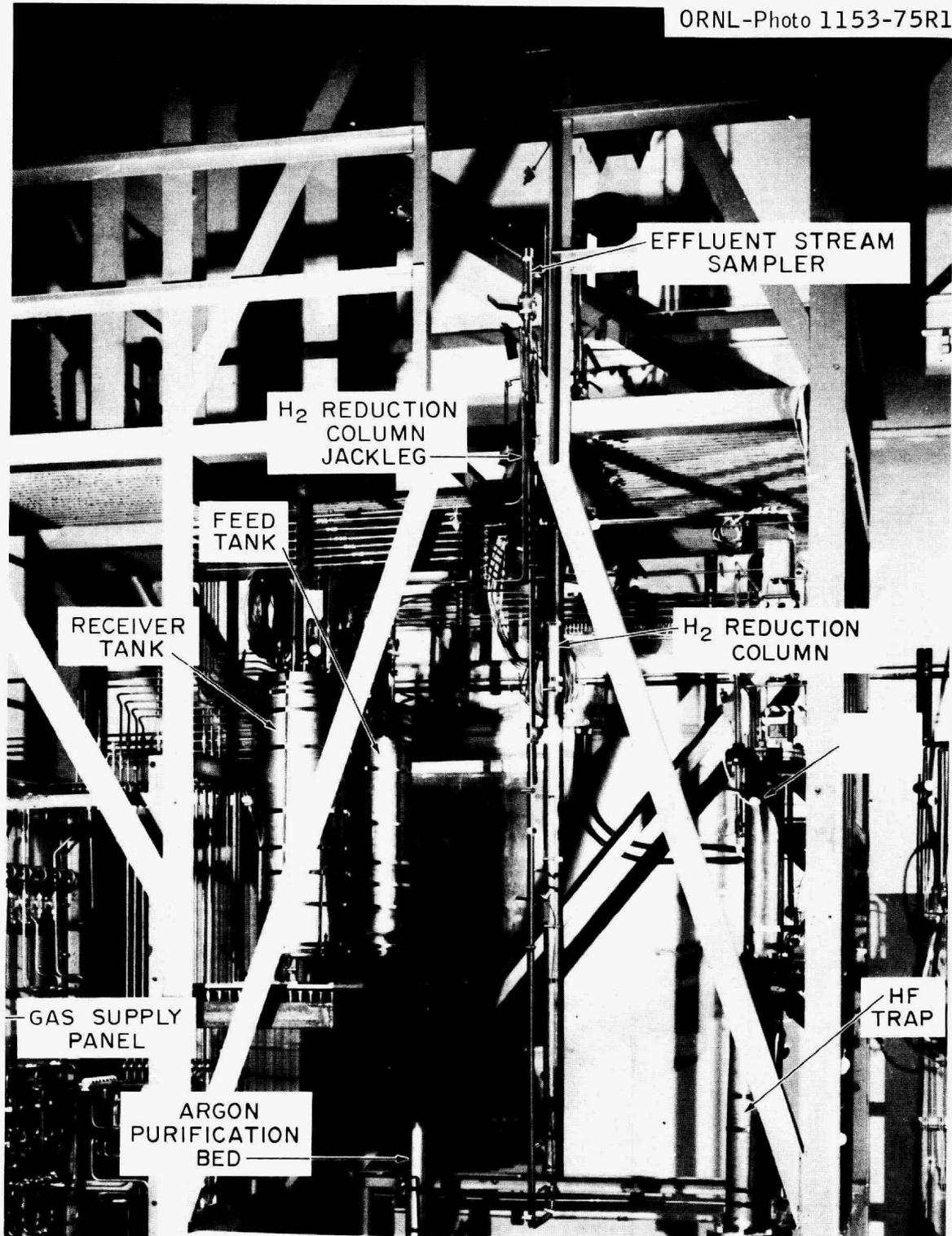
Fig. 11. Overall side view of equipment for Fuel Reconstitution Engineering Experiment before addition of thermal insulation.
