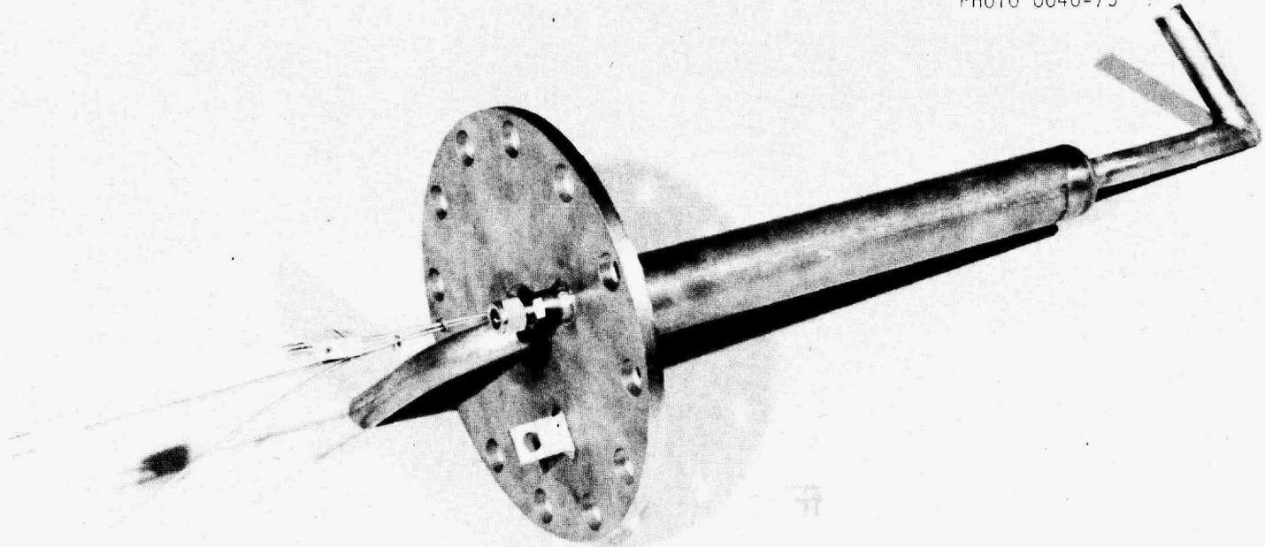
Fig. 4. Electrode to be used in test vessel of autoresistance heating test AHT-4.
