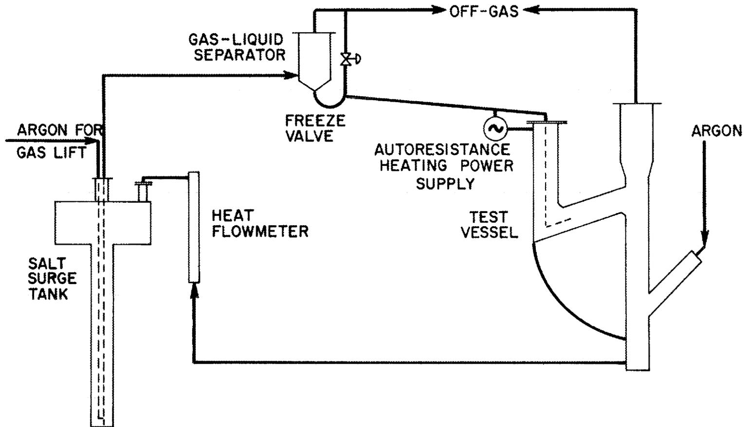
Fig. 1. Flowsheet for autoresistance heating test AHT-4.
