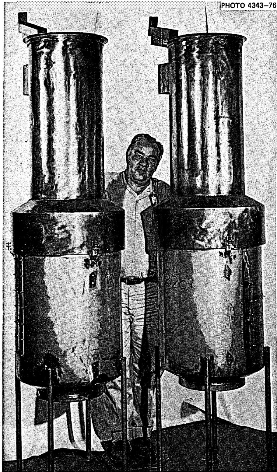
Fig. 13. Cooler housings for corrosion loop FCL-3.
