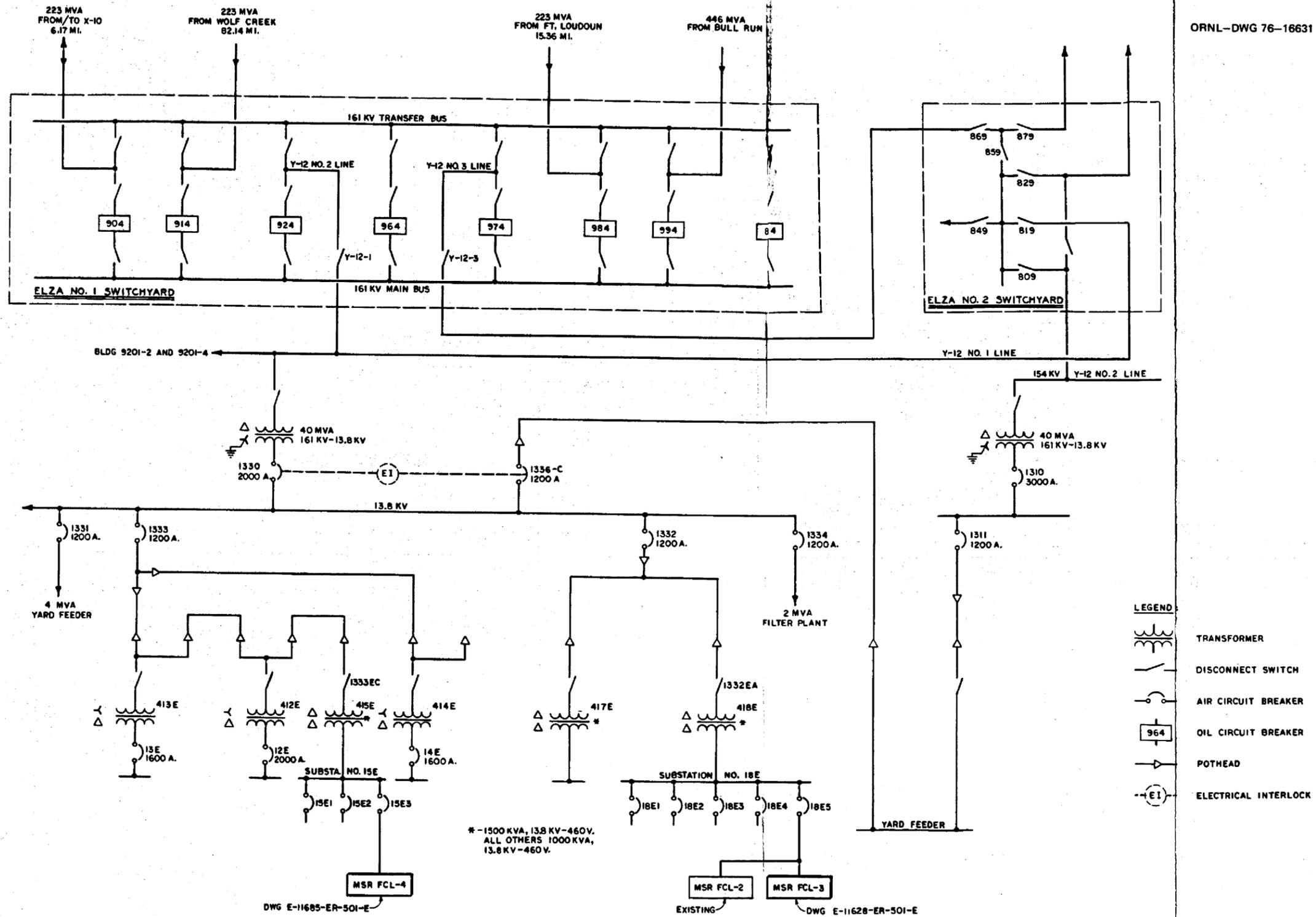
Fig. 16. One-line diagram of area power supply.
