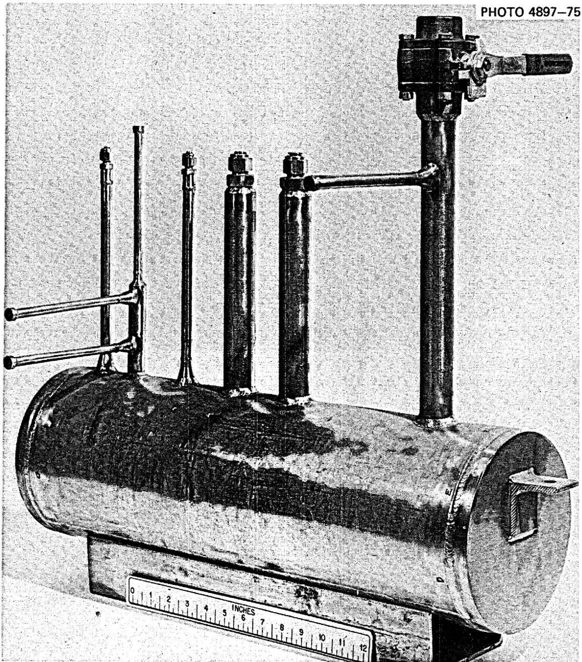
Fig. 11. Fill-and-drain tank for FCL-3 and -4 (1 in. = 25.4 mm).
