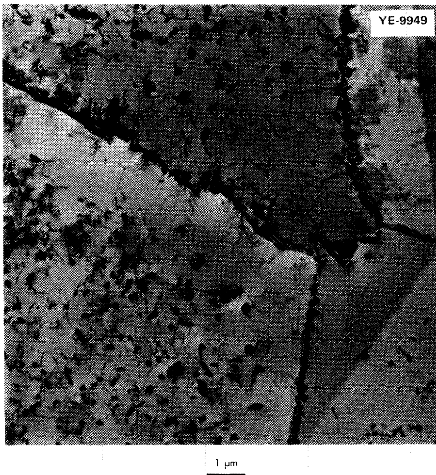
Fig. 1. Typical MC carbide distribution in hafnium-modified Hastelloy N. The alloy contains 0.7% Hf and 0.06% C and was aged 200 hr at 760°C. Original magnification: 5000X.
