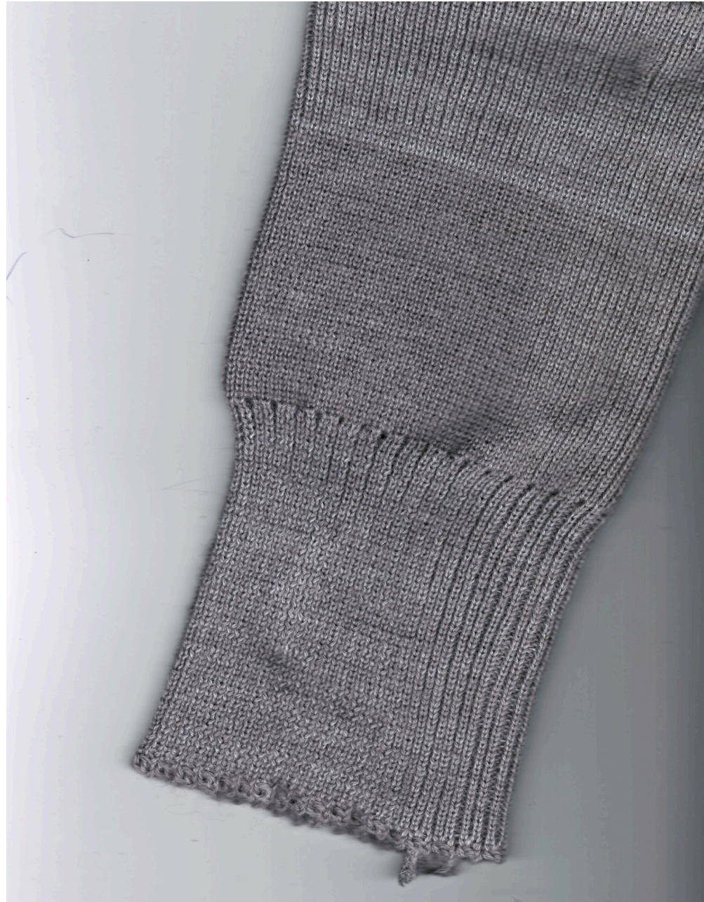
example of a sleeve with added cuffs and piezoresistive yarn.
